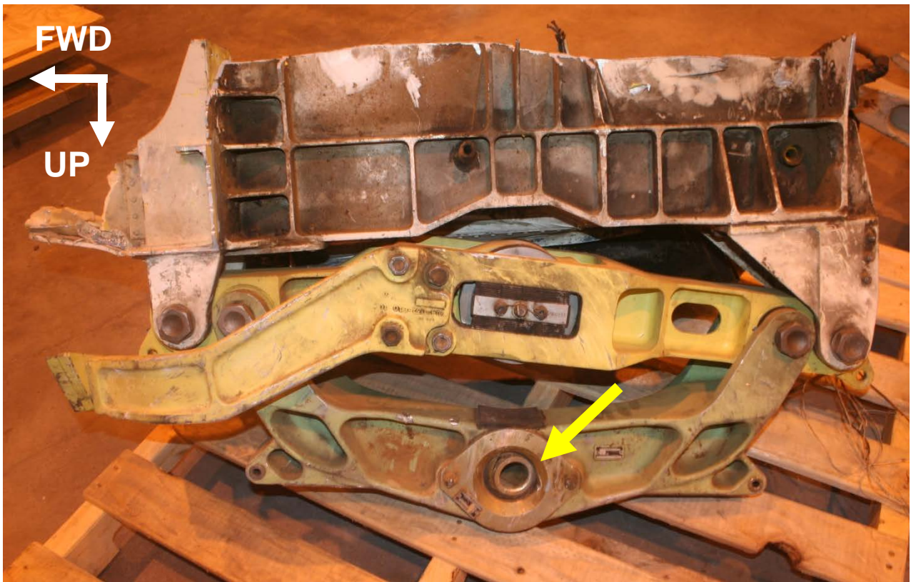
Photo 32. Left nodal beam support assembly for the main transmission. The arrow points to the spherical bearing with the aft-ward bias as recovered.
