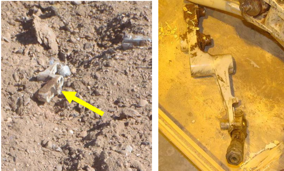
Photo 17. The collective lever arm in a photo taken at the accident site (left image [image courtesy of USTRANSCOM]) and the collective lever arm from the recovered wreckage (right image).
