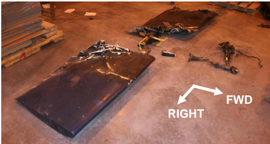
Photo 29. Recovered pieces of the elevator system.
