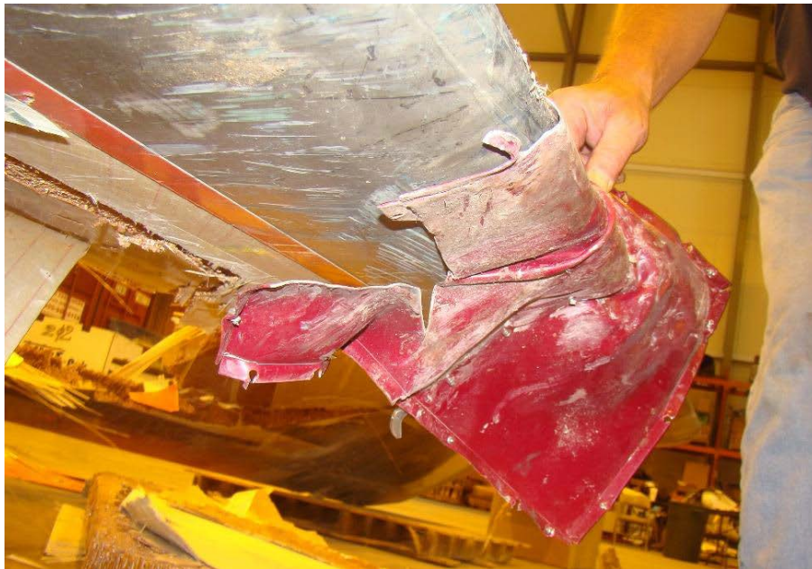
Photo 7. Deformed helicopter battery cover (placed over the ‘red’ main rotor blade leading edge).
