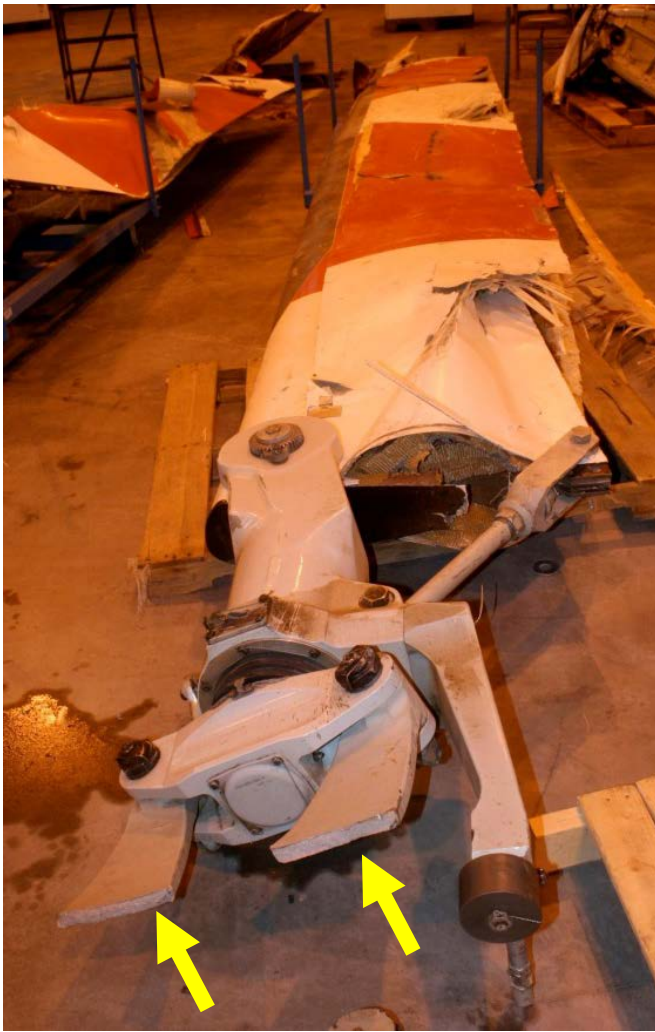
Photo2. The red main rotor blade. Arrows indicate yoke flange fractures.
