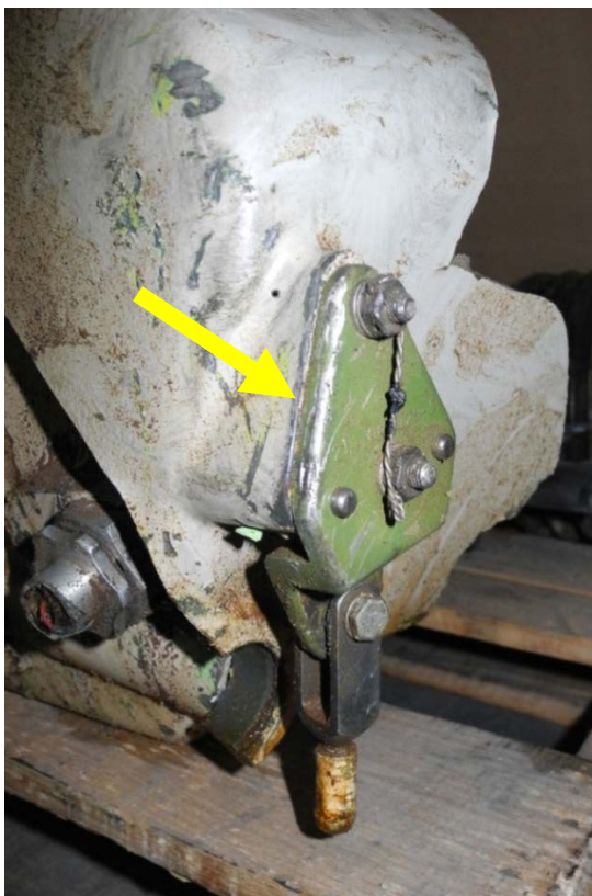
Photo 21. Isolation tube mount and clevis connection on the main transmission sump case.
