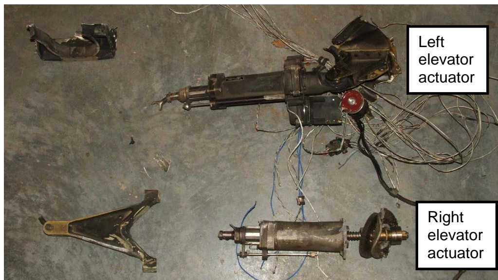
Photo 30. Left (top) and right (bottom) elevator electrical actuators.
