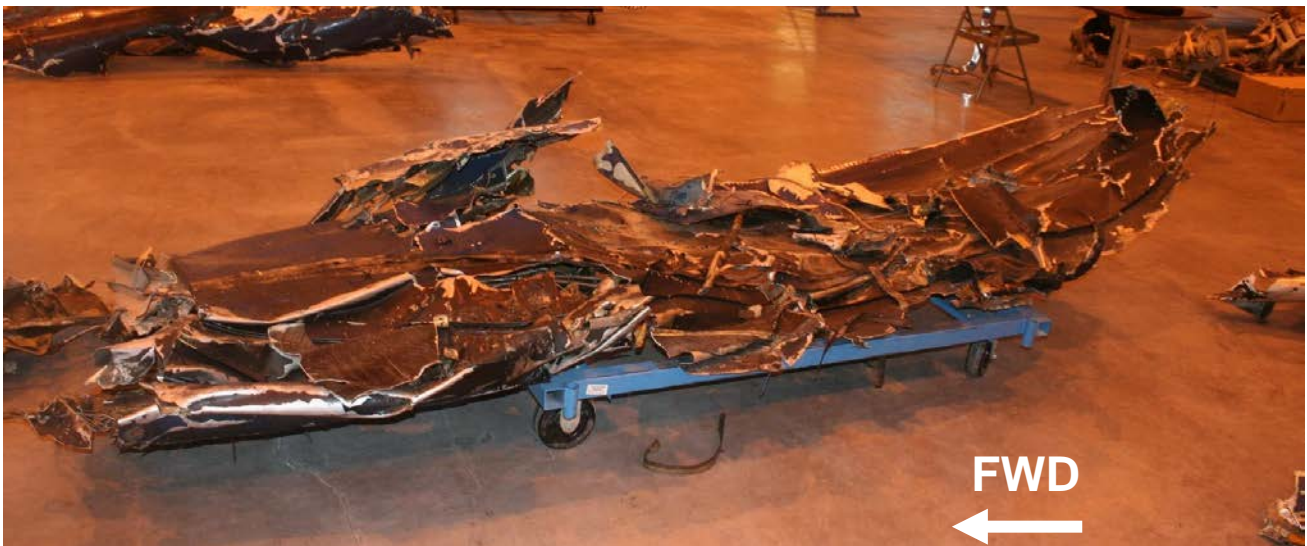
Photo 39. The recovered forward tailboom section (left-side outer skin is visible).
