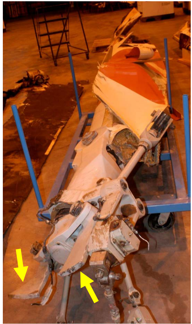
Photo3. The white main rotor blade. Arrows indicate yoke flange fractures.
