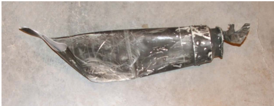
Photo 37. A severed section of tail rotor drive shaft.
