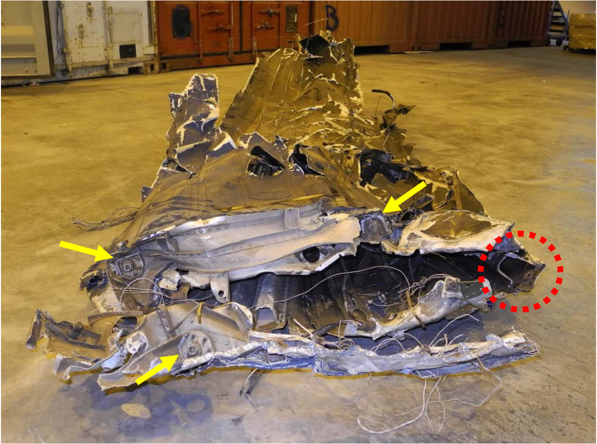
Photo 42. Three of the four tailboom attachment fittings with attaching hardware present (yellow arrows) and the fractured fourth attachment point (red circle).
