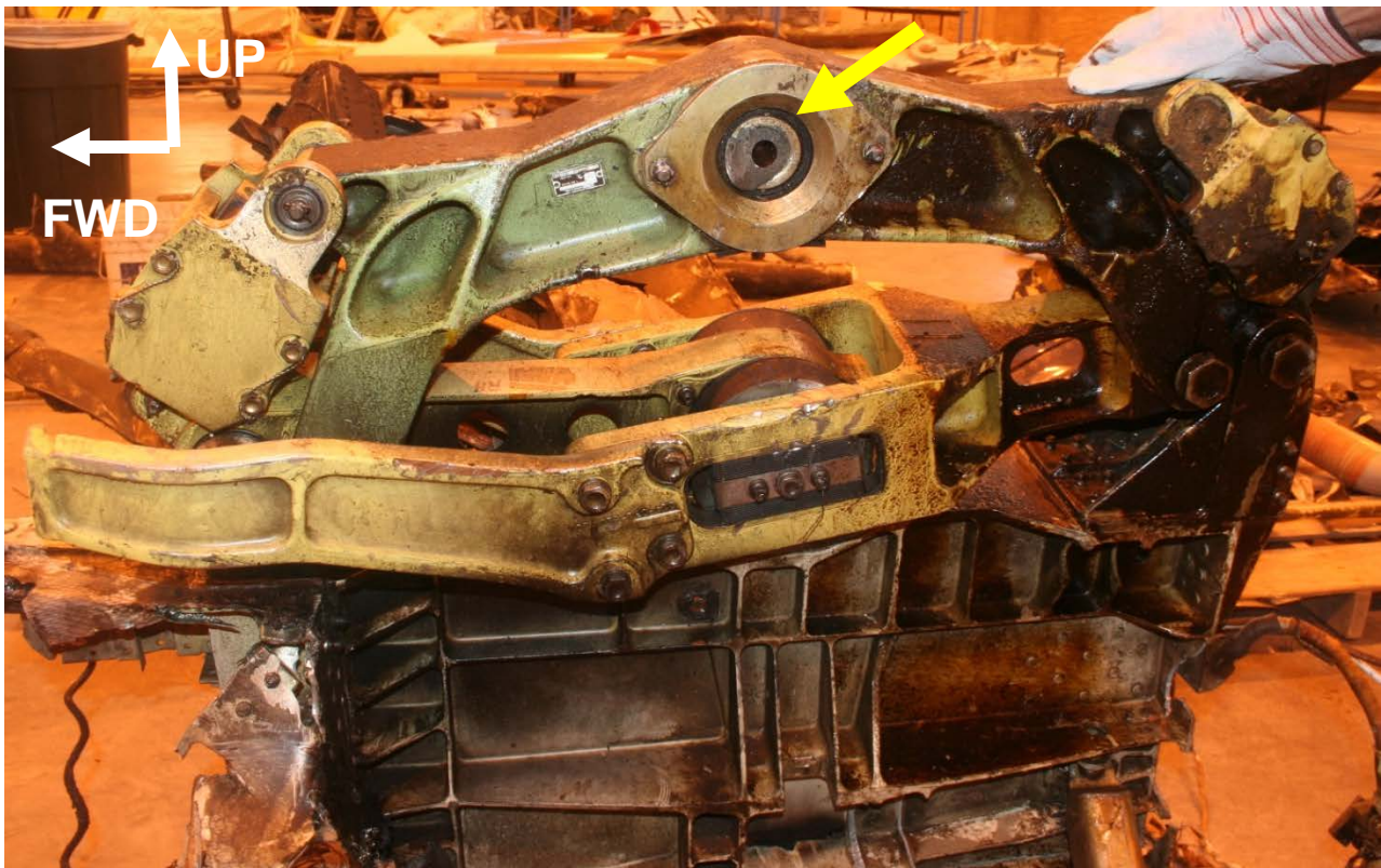
Photo 33. Right nodal beam support assembly for the main transmission. The arrow points to the fractured portion of the transmission mounting spindle found within the spherical bearing.
