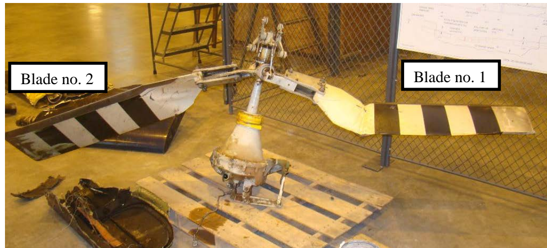
Photo 38. Tail rotor gearbox with tail rotor blades installed.
