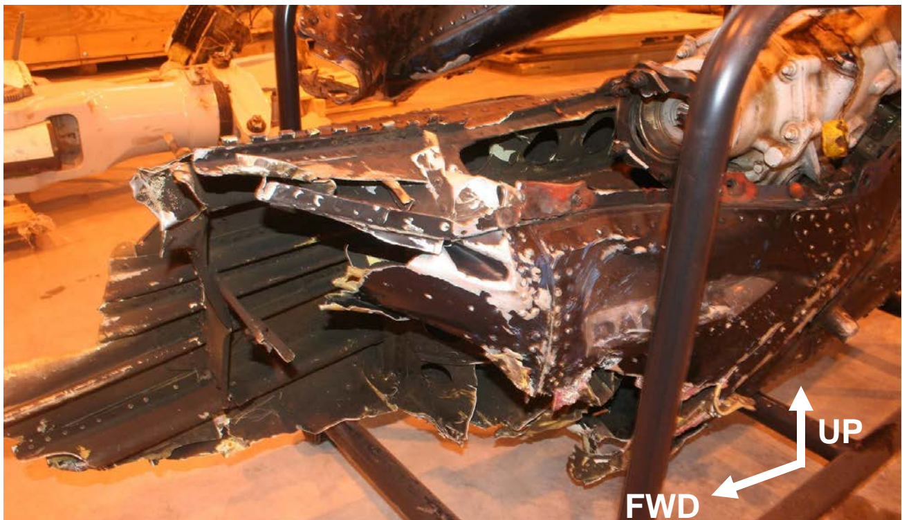
Photo 40. Forward section of the severed tailboom and vertical fin.
