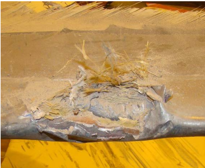
Photo 5. The white main rotor blade's leading edge abrasion strip with missing piece.
