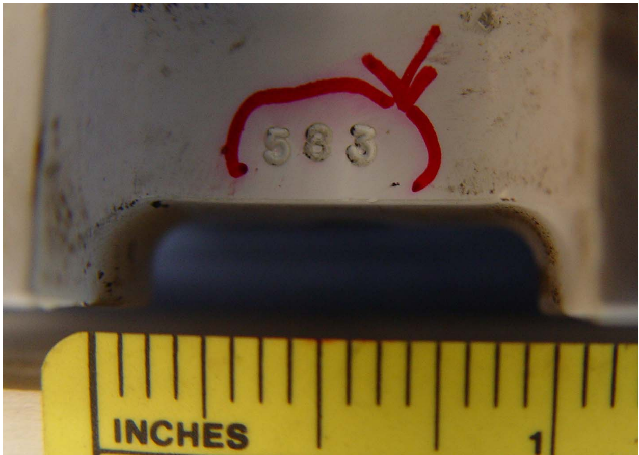
Figure 10 – Incident NLG End Cap serial number stamp
