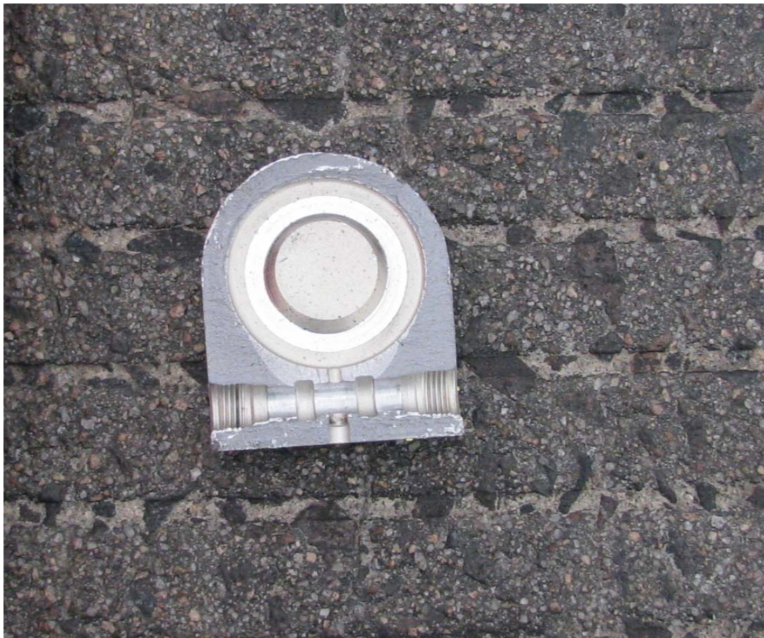
Figure 2 – NLG End Cap piece found on runway
