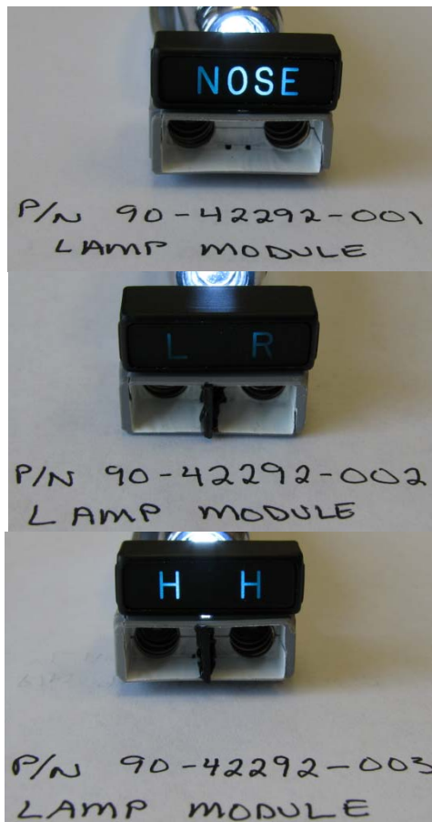
Figure 8 – Landing gear position annunciator lamp modules
