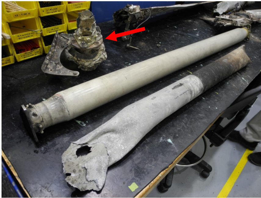
Photo 21. The No. 4 TRDS (bottom shaft), No. 5 TRDS (top shaft), and unlabeled TRDS airframe mount (red arrow).
