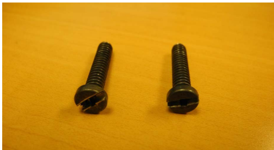
Photo 26. Replicated modified compression screws used for testing at Bell Helicopter Broussard.
