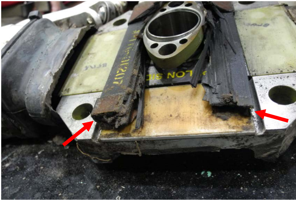
Photo 11. The fracture observed at the ‘yellow’ tail rotor blade spar.
