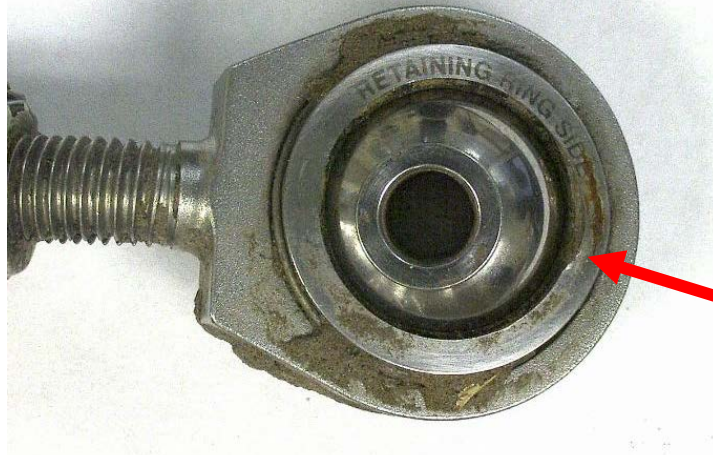
Photo 7. Trunnion impact mark 180° opposite of the trunnion impact mark seen on opposing side of the ‘yellow’ PCL blade-side rod end. [photo courtesy of SAC]
