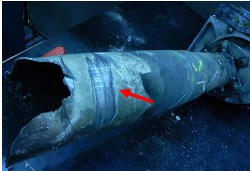
Photo 22. The No. 4 TRDS with the rotational smear marks near the fracture. [photo courtesy of SAC]
