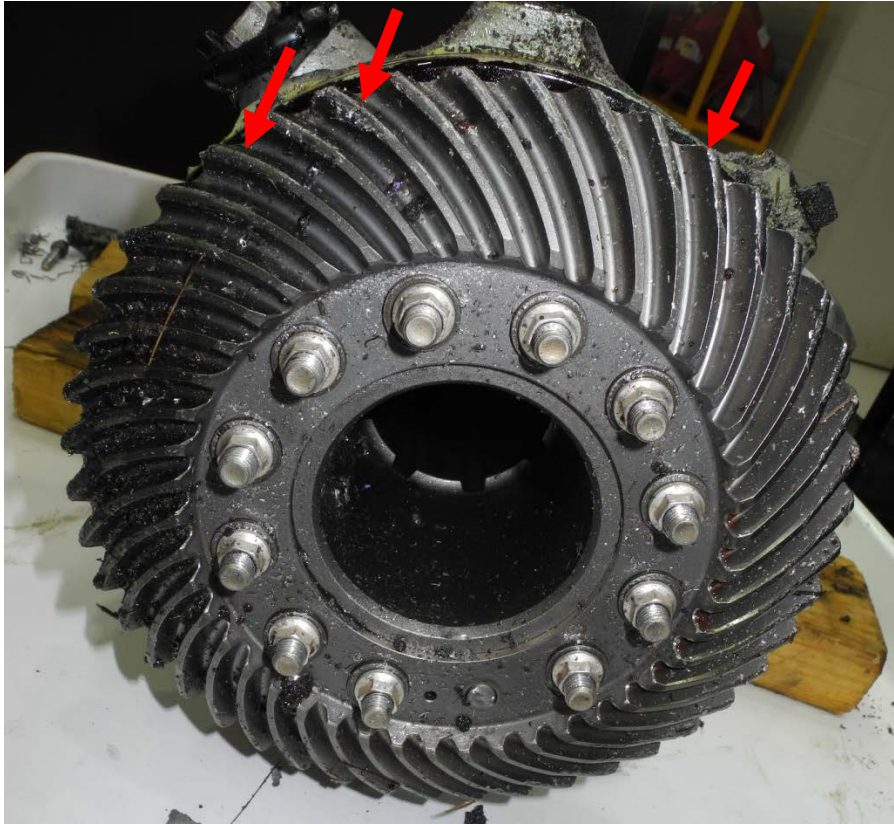
Photo 15. Damage seen on the top lands of the output bevel gear teeth.
