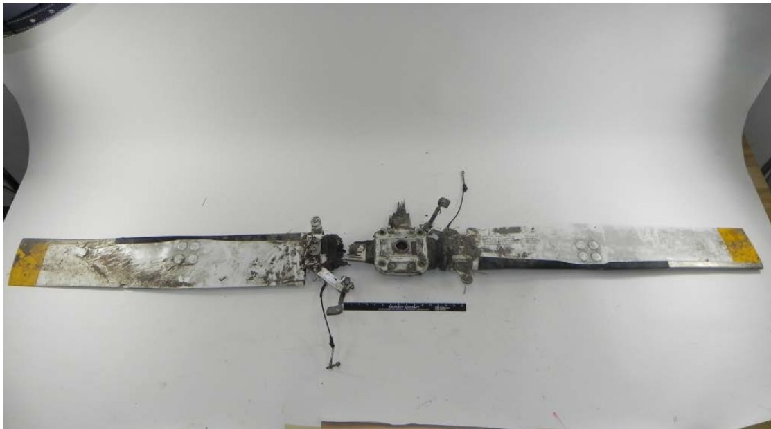
Photo 13. Overall view of the 'black' (left) and 'blue' (right) tail rotor blade. The outboard retention plate and the remnant 'red'/'yellow' spar is seen in the center. [photo courtesy of SAC]
