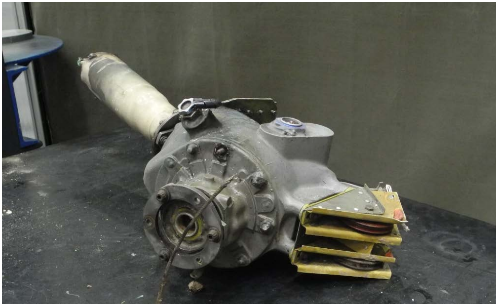
Photo 23. The recovered IGB as received. The No. 4 TRDS remains attached to the input flange.
