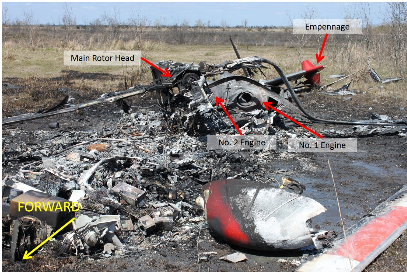
Photo 1. N574EH at the accident site exhibiting heavy damage from the post-crash fire.
