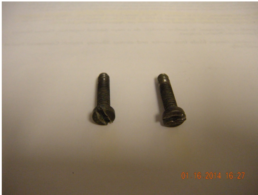
Photo 25. Modified compression screws used at Bell Helicopter Broussard. [photo courtesy of BHTI]
