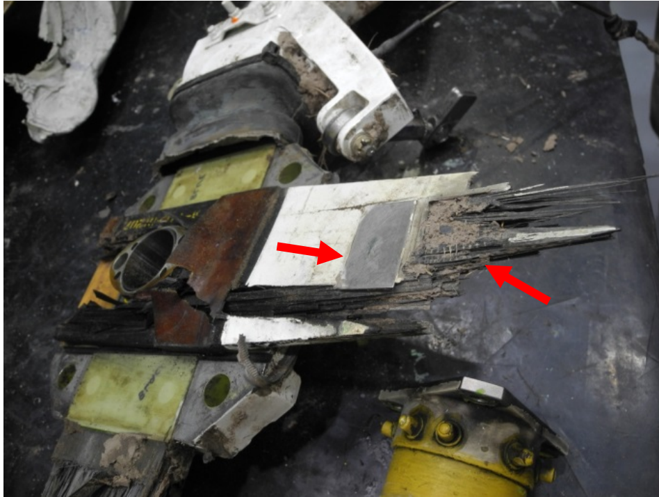
Photo 10. The spar fracture for the 'red' tail rotor blade. The left arrow points to the bumper plate and the right arrow points to the remnant adhesive layout for the pivot bearing retainer.
