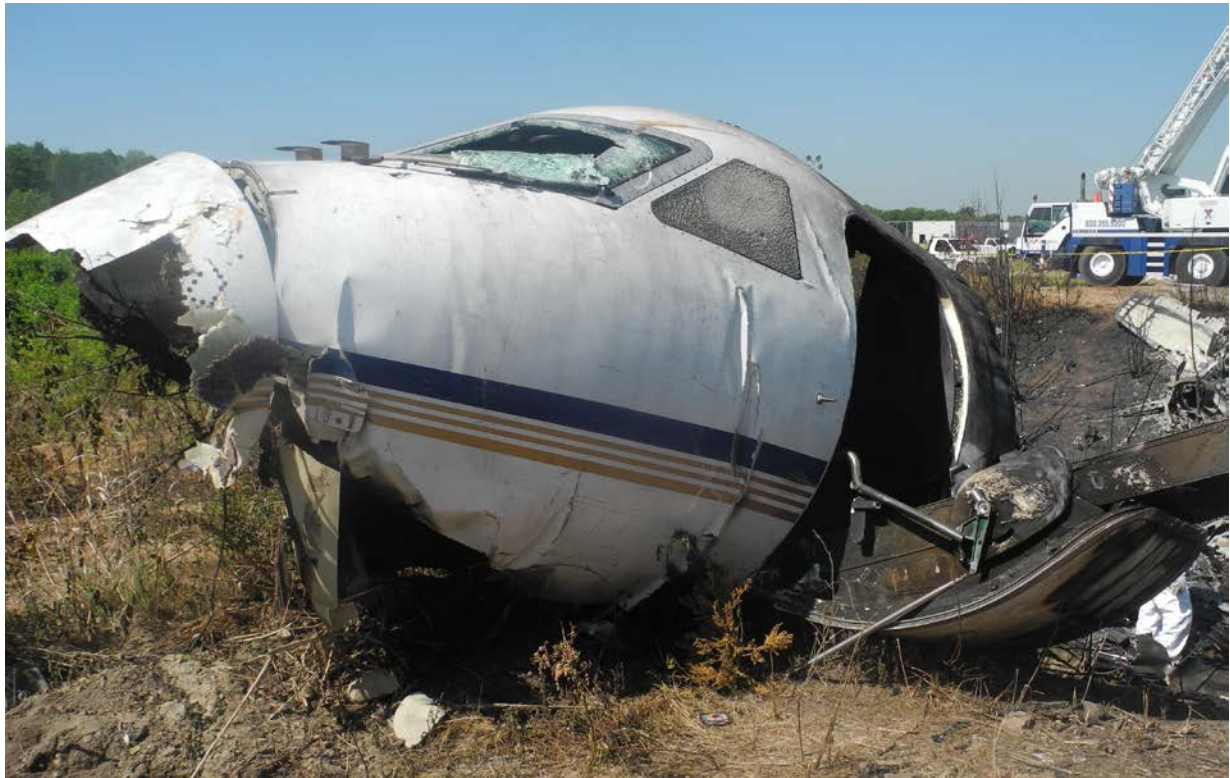
Figure 4: Forward Fuselage Structure
