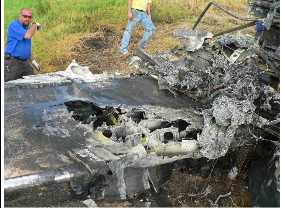
Figure 16. Bottom of the left wing, shown during recovery, exposing the leading edge opening into the fuel tank that aligned with the path past the concrete post on the west side of the roadway.
