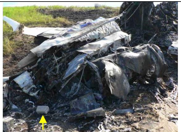
Figure 20. Right aft fuselage and engine. Note: The arrow points to the top of the concrete marker post from the west side of the road.
