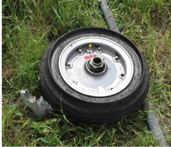
Figure 21. Nose landing gear tire and yoke assembly, resting on the east side of Highway 302. The pole is a fence post from the west side of the highway.
