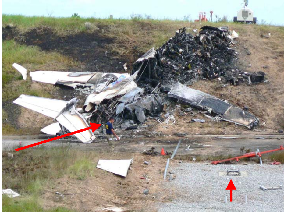
Figure 8. Airplane wreckage as viewed from mid-way down the slope, between the runway safety area and the approach light pole. The base of the broken light pole is at the lower right arrow. The arrow at the lower left points to the base of the broken concrete roadway right-of-way (R/W) marker and where the top was found (See also Figure 18). The fuel-burned area begins at the post.
