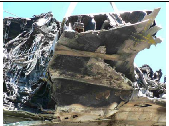
Figure 18. The right main landing gear well from below. The indented leading edge along the right edge of the photo better shows where the succession of three airport perimeter fence posts struck.
