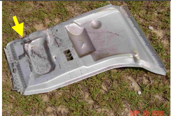
Figure 27. Right main landing gear door with impacts along the trailing edge (arrow) and black rubber transfers near the hinge.
