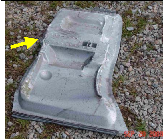
Figure 26. Left main landing gear door with impacts along the trailing edge (arrow) and black rubber transfers near the hinge.
