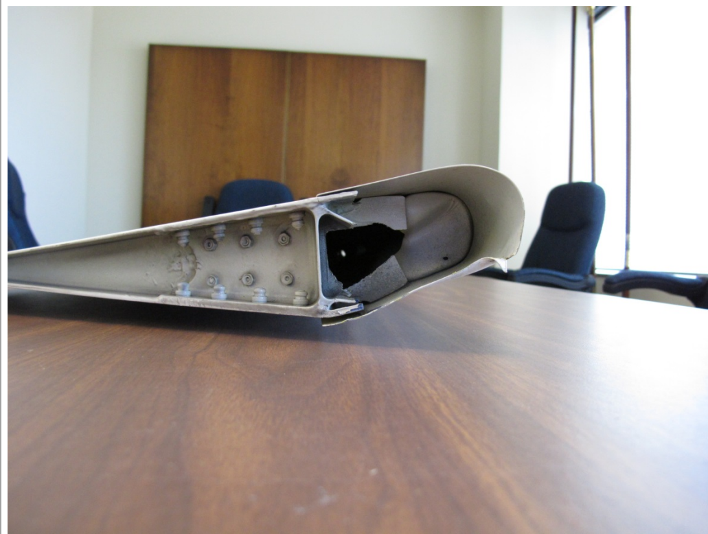
Left elevator root - torque tube structure & separation fracture surfaces.
