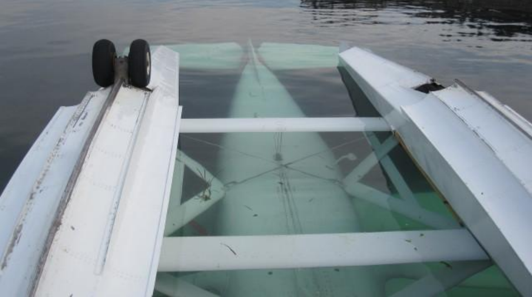
Airplane, Bottom View Showing Extended Aft Gear. FAA Photo.
