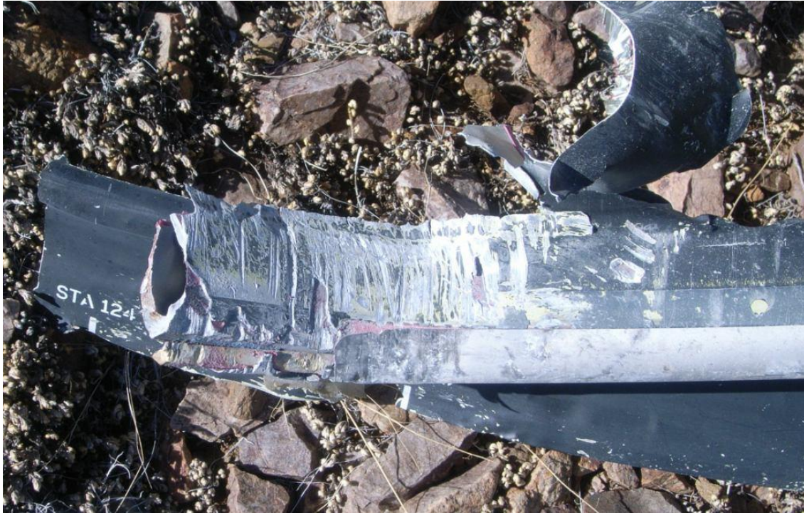
Figure 13 - Segment of Main Rotor Blade with Chordwise Scoring
