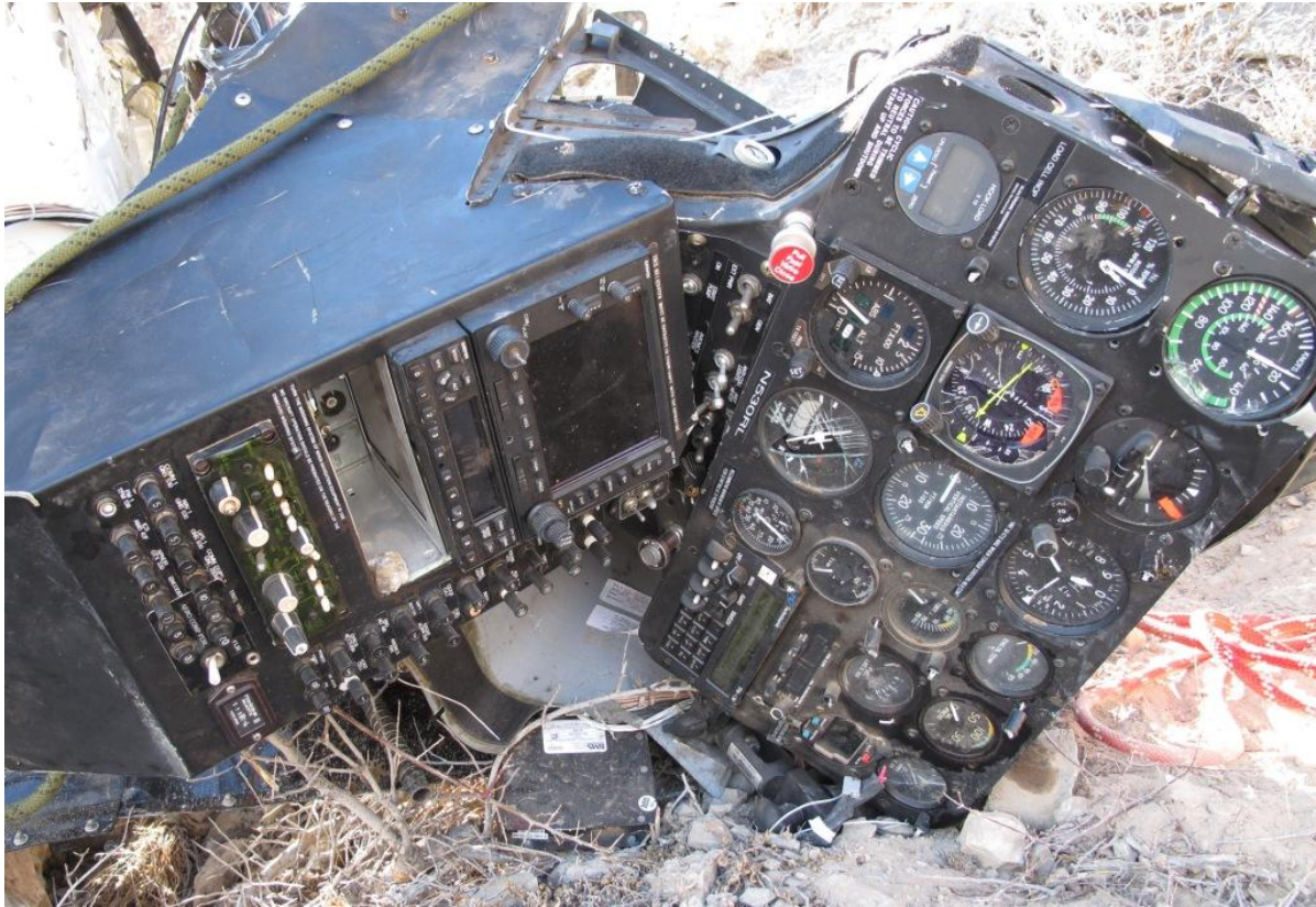
Figure 9 - Two-Segment Instrument Panel Outside Helicopter
