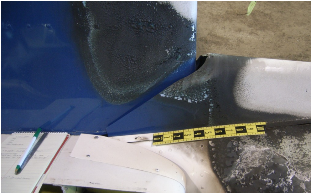
Figure 4 - Fin LE to Fairing Gap
