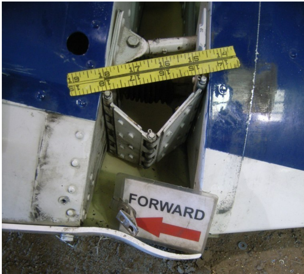
Figure 5 - Empennage Hinge Measurement Geometry
