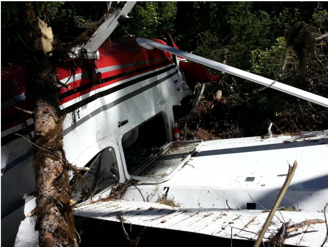
Figure 4 - Left Side of Fuselage (note flap extension angle)
