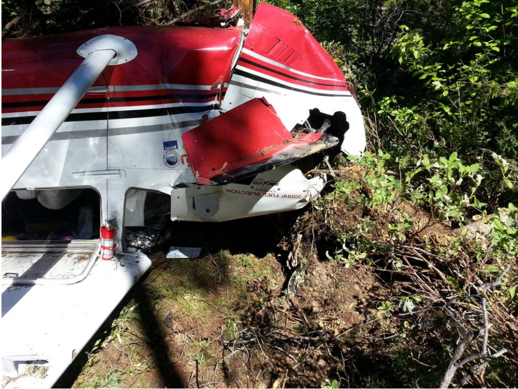
Figure 3 - Forward Fuselage and Ground Impact Location
