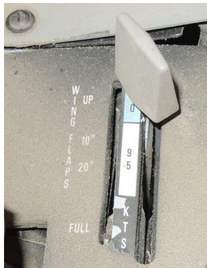
Figure 18 - Flap Control and Indicator
