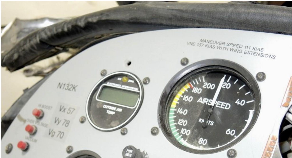
Figure 14 - Airspeed Placards/Notations (note VNE discrepancy)
