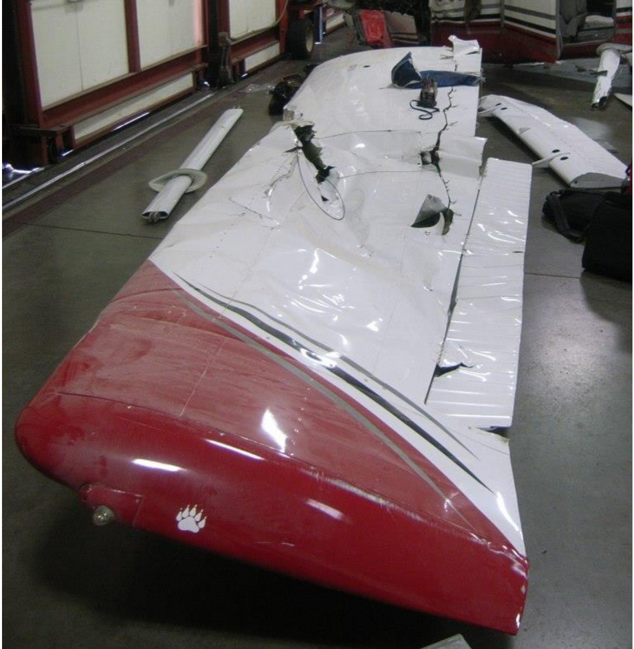
Figure 7 - Left Wing (note aileron crossover cable tear-out)
