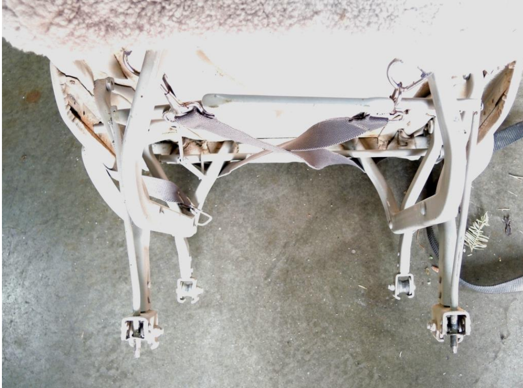
Figure 10 - Copilot Seat Feet (seat unoccupied for accident but separated from tracks)
