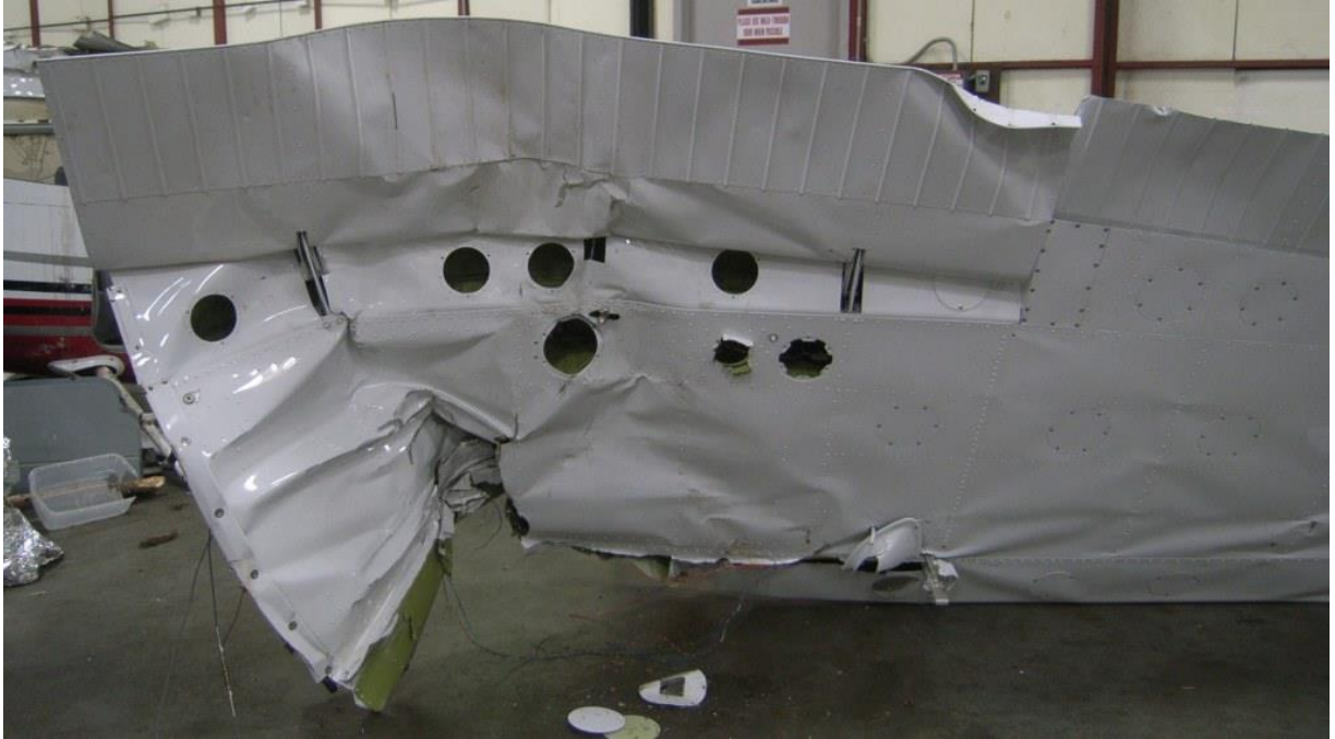
Figure 20 - Right Wing (separated at impact)
