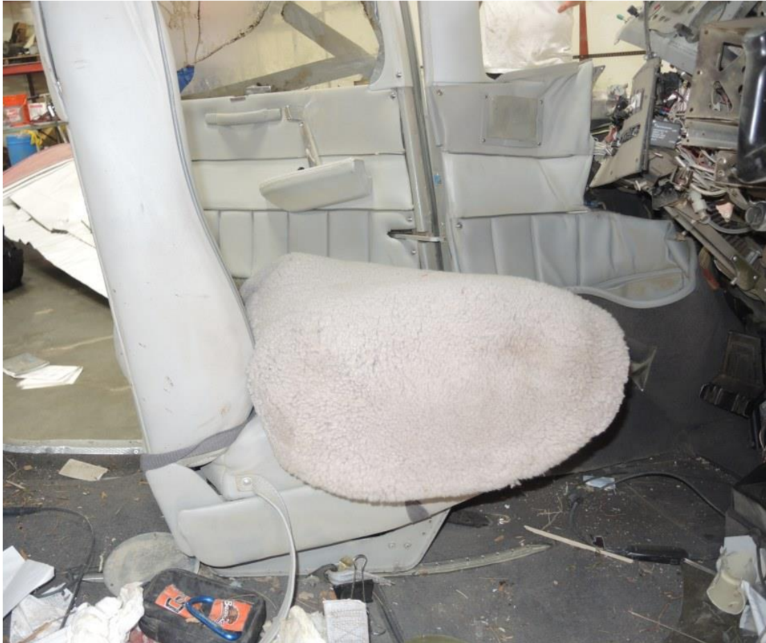
Figure 9 - Pilot's Seat (note cabin integrity, plus deformed seat tracks)
