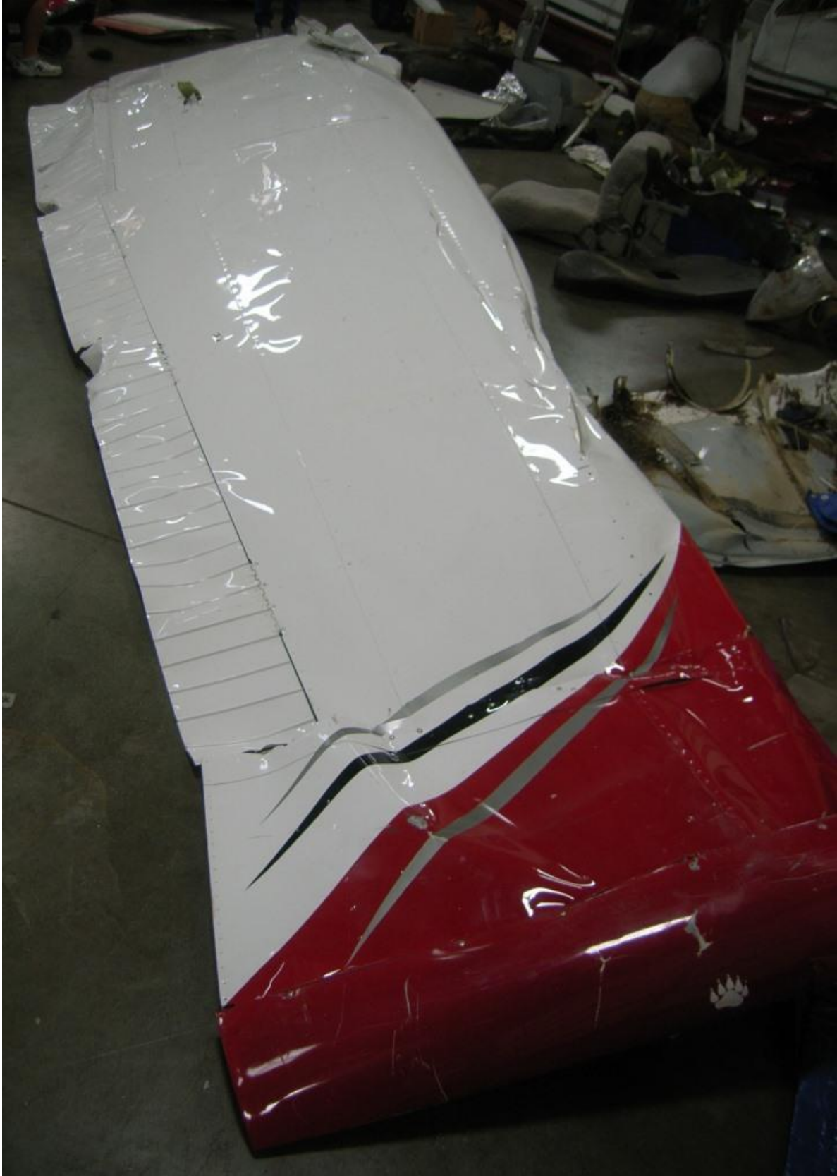
Figure 8 - Right Wing (separated at impact)
