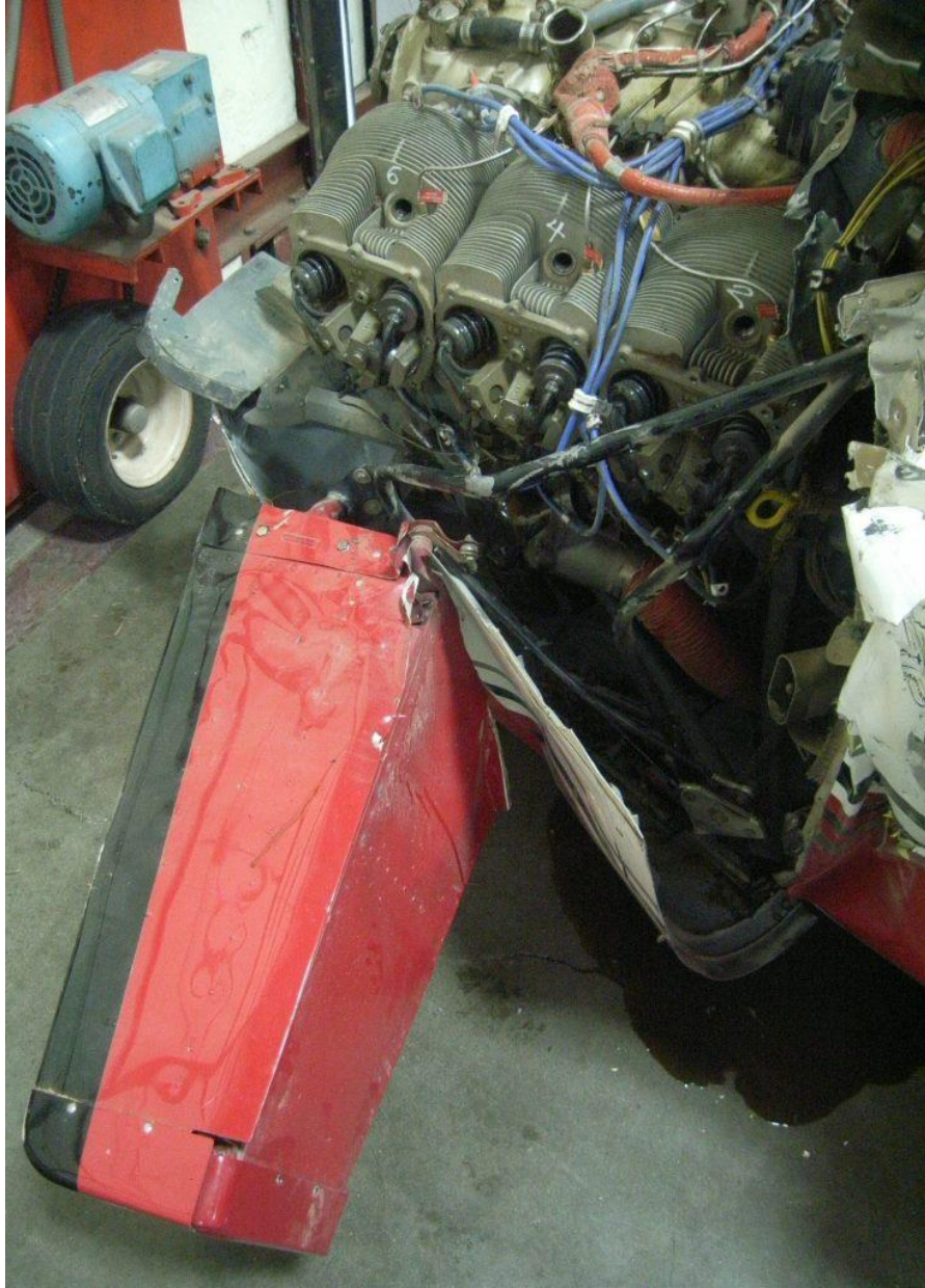
Figure 22 - Left Canard (outboard end displaced aft)
