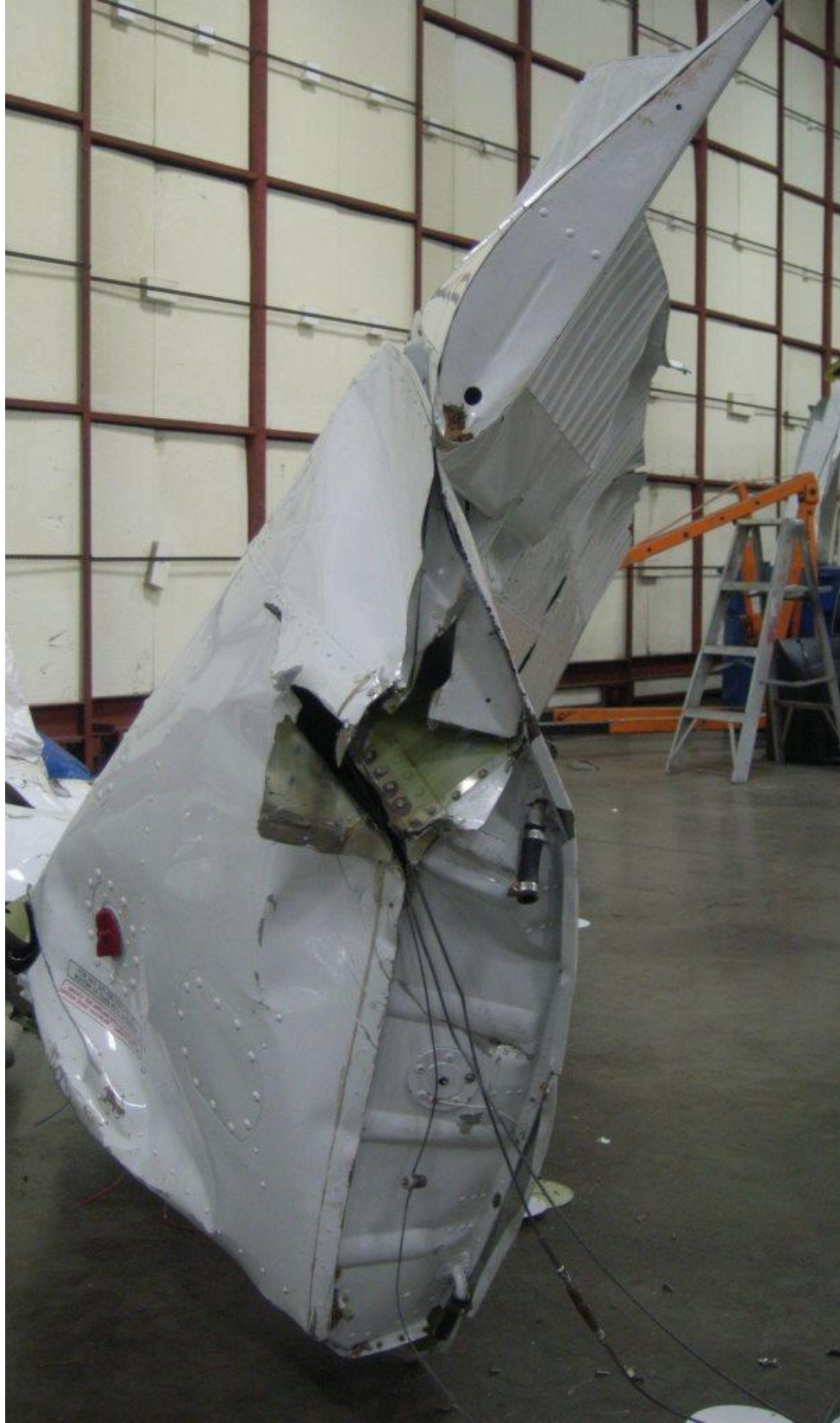
Figure 19 - Right Wing Root (note flap deflection)
