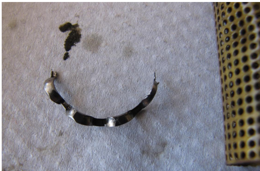
Figure 3: Piece of the left magneto bearing retainer cage
