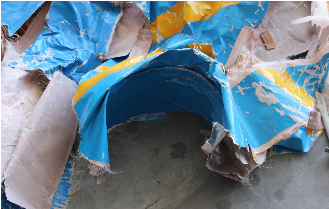
Figure 2: Lower left wing impact damage
