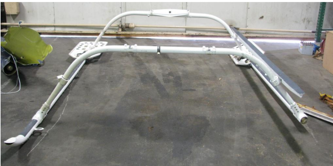
Figure 5 - Front View of Skid Assembly (removed for recovery)
