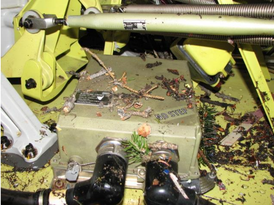
Figure 25 - Engine Control Unit (ECU) Before Removal
