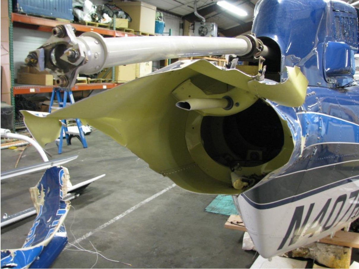
Figure 12 - Tailboom/Fuselage Fracture (Note TR drive shaft)
