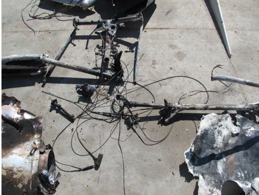
Photo 3 Cockpit Flight Control Components and Cables
