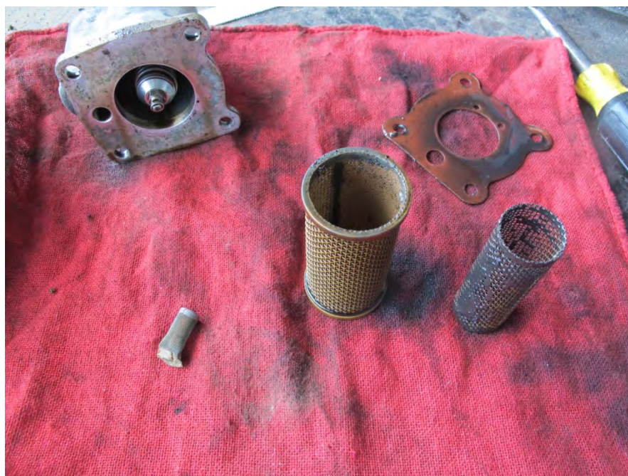
Photo 13 Oil Suction and Oil Pressure Screens
