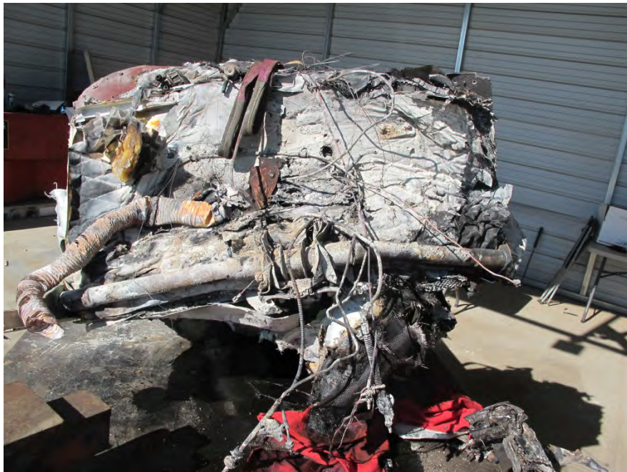
Photo 2 Cabin Area Aft of Firewall
