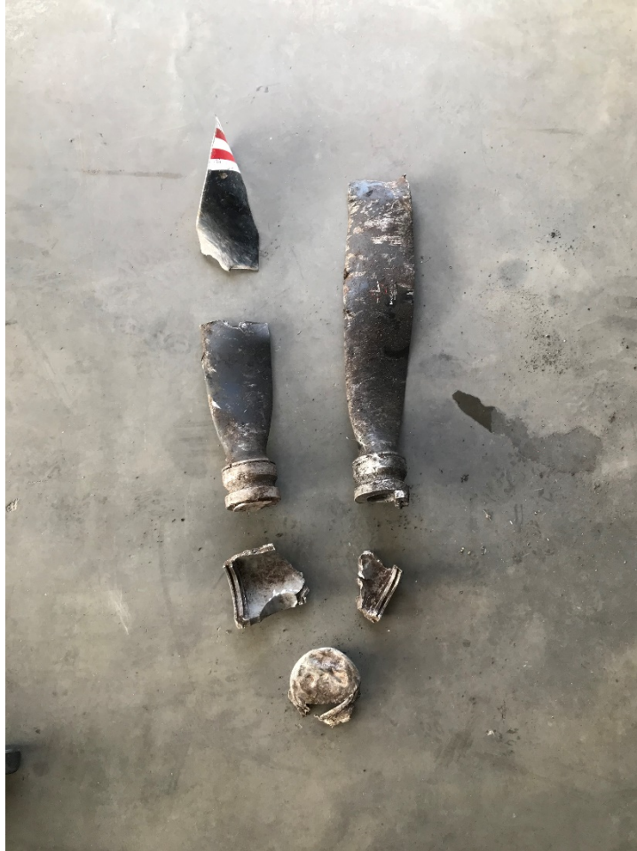
Figure 18: Propeller Blades, Hub Fragments, and Front of piston cylinder
