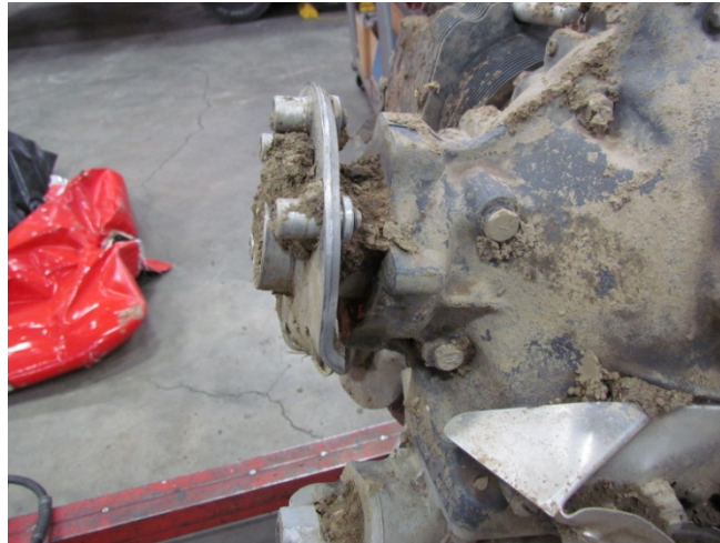
Figure 4: Bent Propeller Flange
