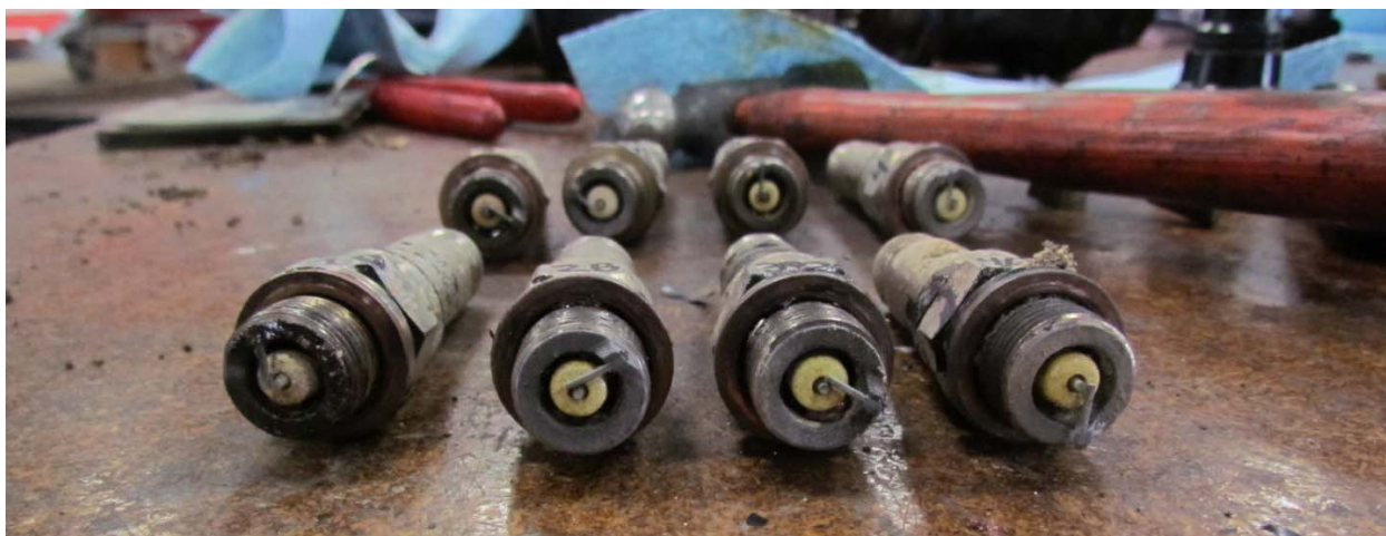
Figure 3: Spark Plugs (the forward plugs are the bottom spark plugs; the aft plugs are the top spark plugs)
