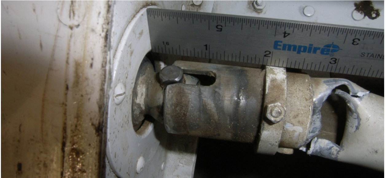
Figure 16 – Improper/Incomplete Fit of Left Wing Air Brake Control Connection
