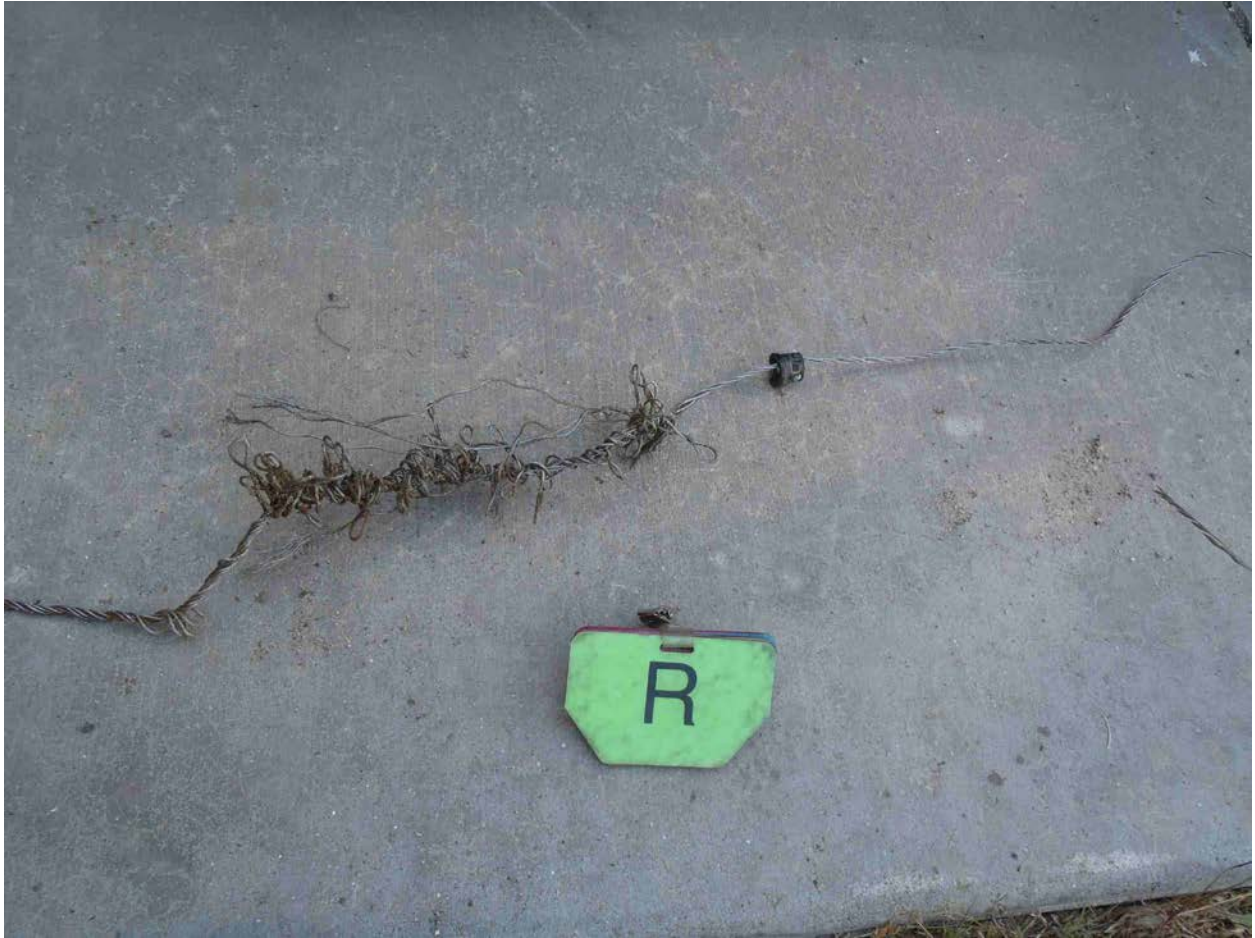
Photo 12 - Aileron Balance Cable, Right Side
