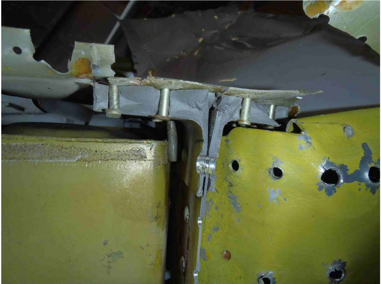
Photo 9 - Left Wing Spar Cap Fracture Surface
