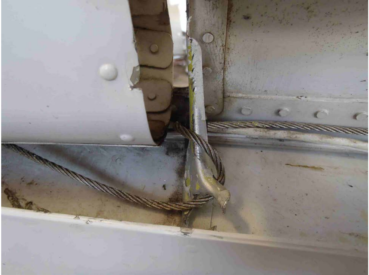
Photo 11 - Left Wing Aileron Cable
