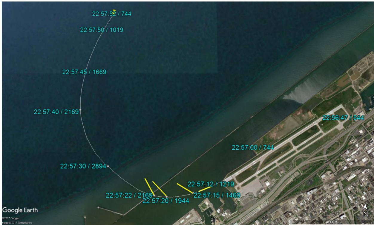
Figure 8. Selected heading shown as yellow lines at time of change/selection. The yellow line points towards the heading selected and intersects the flight path at the point in time when it was selected.
