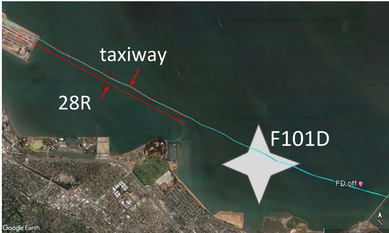
Figure 11. Airplane track with approach tracks to 28R and taxiway C. F101D is shown at the scale of FMS Bridge Visual Runway 28R chart.
