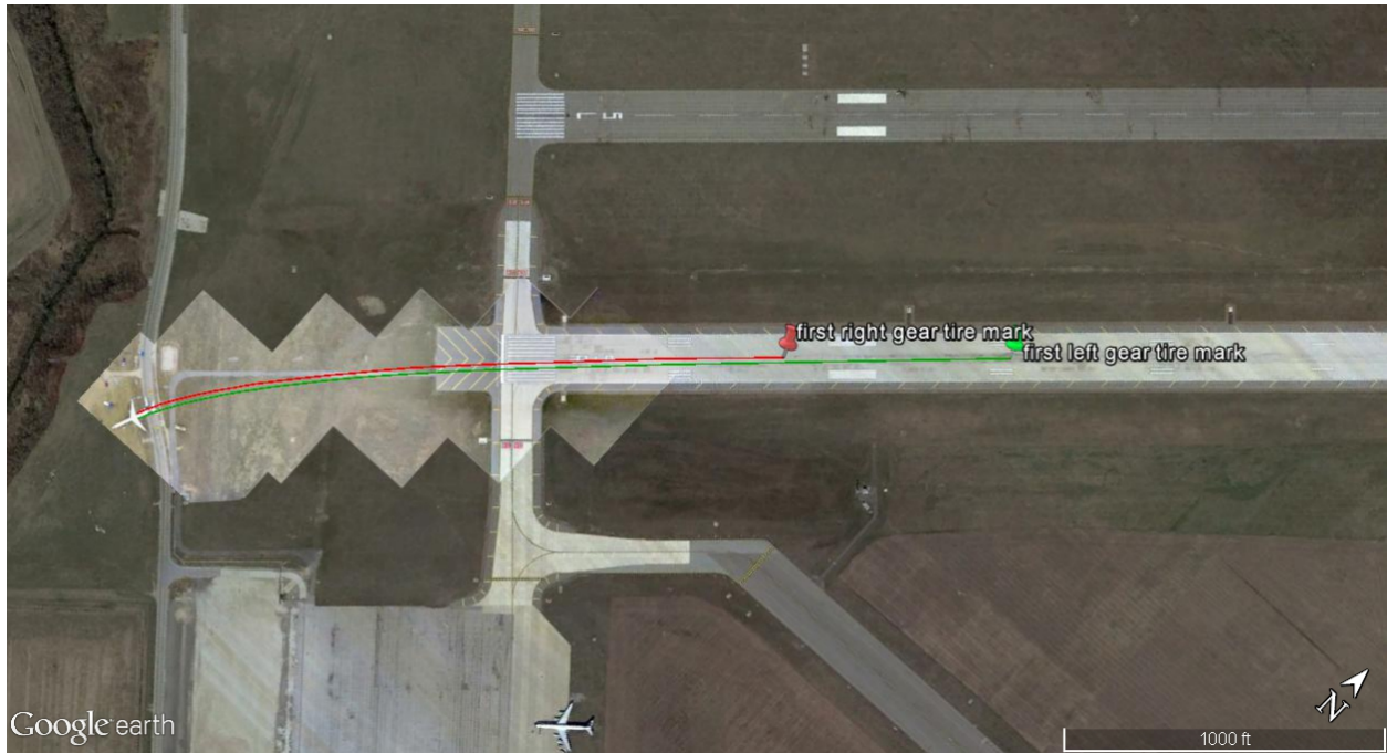
Figure 1. End of runway 23L, left and right main gear tire marks are highlighted green and red, and the airplane's final position can be seen.
