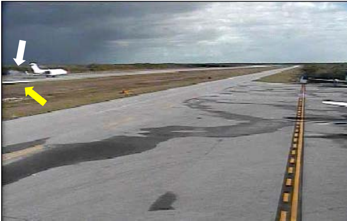
Figure 5. Security camera still from MKY of the accident aircraft on runway. The white mark to the extreme left behind the aircraft is the 1,000 ft mark (yellow arrow). The small cloud of smoke behind the aircraft (white arrow) visible in this frame was indicative of touchdown.
