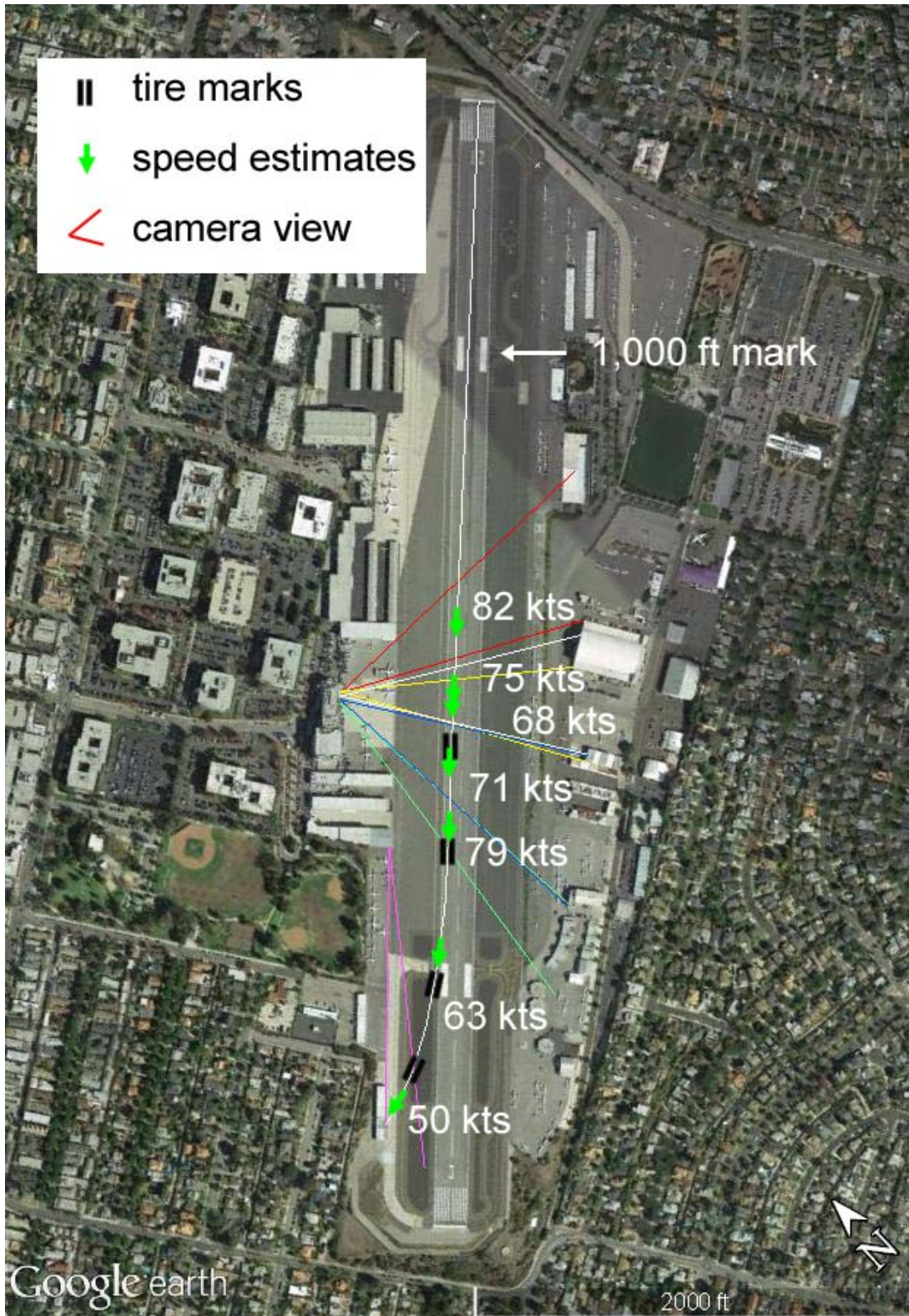
Figure 5. Recorded tire marks shown (not to scale) in black. Speed estimates from the Video Study are shown in knots next to green arrows. The projected ground roll path is shown as a white line. The arc of the camera views are shown as colored lines.
