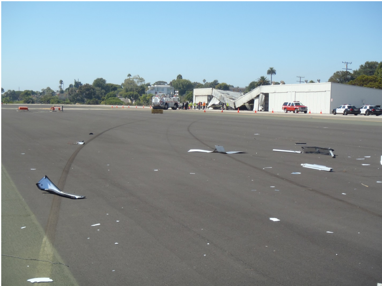
Figure 4. Tire marks from the left and right main gears. The nose gear mark is lighter and closer to the right main tire mark. The hanger the aircraft impacted is in the top right of the picture.
