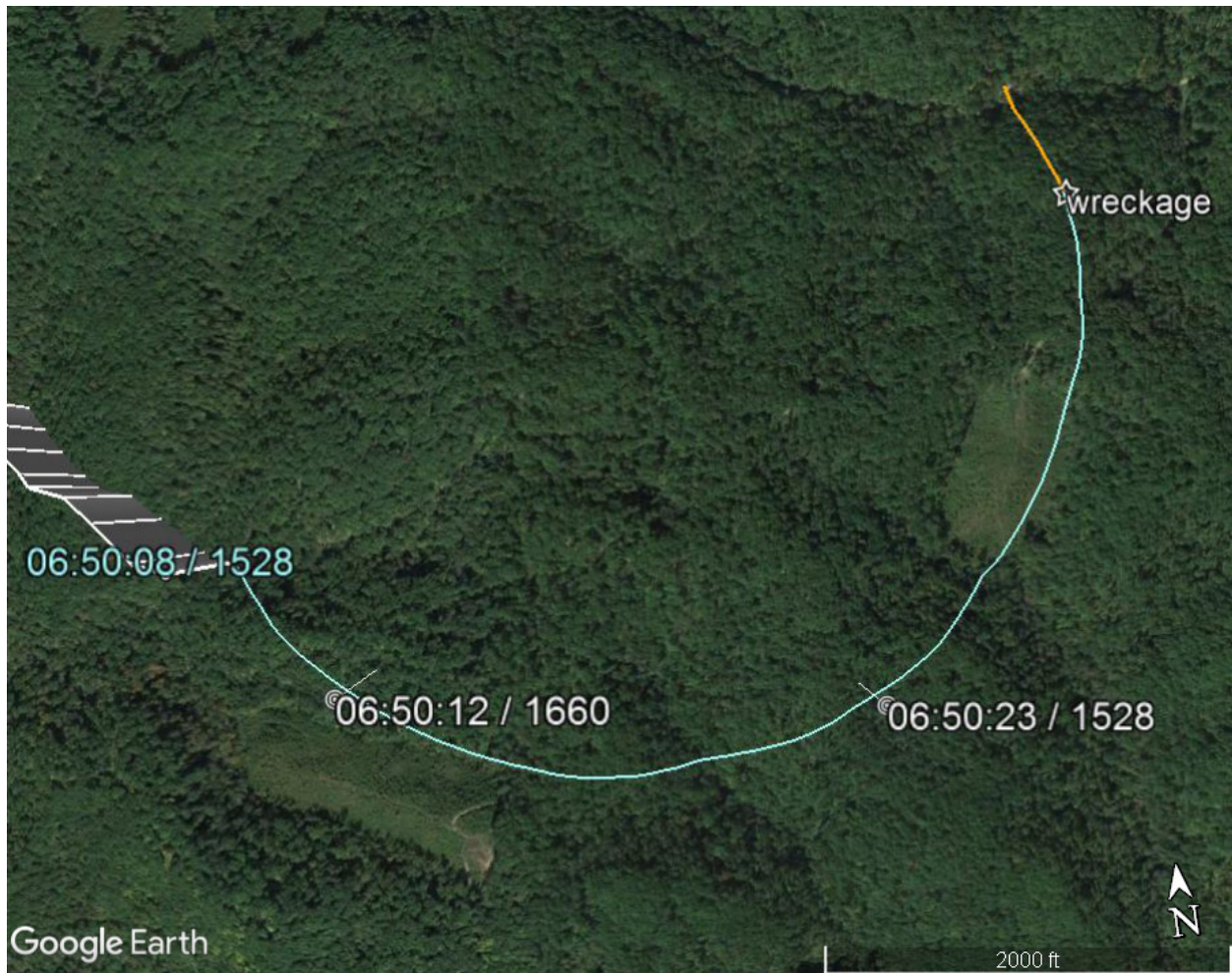
Figure 9. End of flight path, wreckage location, and debris field orientation (orange line).
