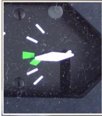
**Figure 19.** Cockpit trim indicator showing horizontal stabilizer position consistent with condition of stabilizer actuator found in wreckage, per Reference 5. Green trapezoid (“sector”) = neutral position; green diamond = takeoff position. Simulation stabilizer set constant at neutral position.
