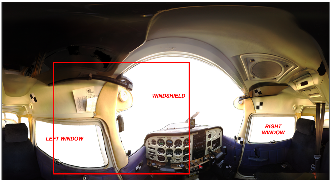
"Fish eye" photograph of the cockpit of an exemplar Cessna 172. The highlighted area is plotted in Figure 20a.
