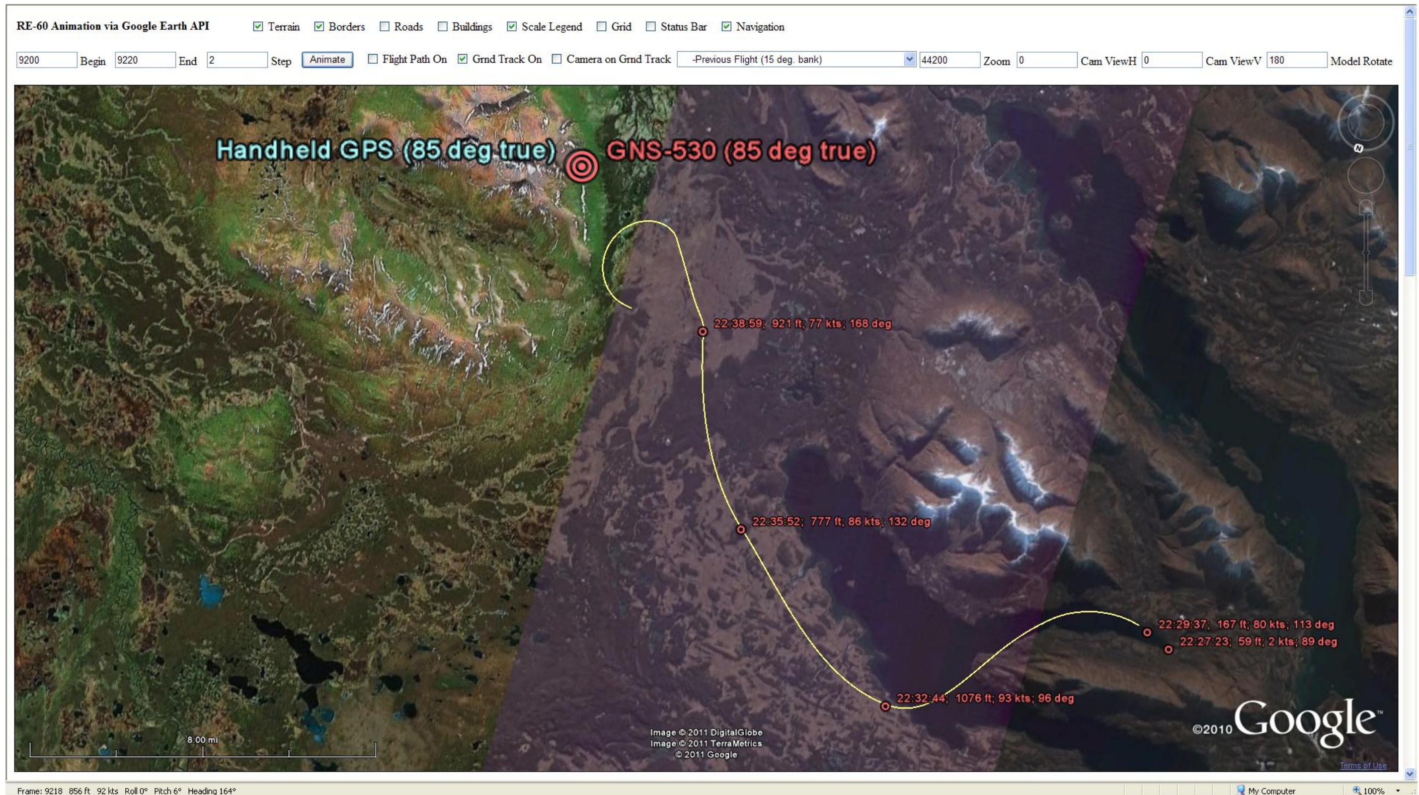
Figure A6.4: N455A simulation scenario 4 (target PREVIOUS FLIGHT waypoint followed by 15° LWD escape maneuver).
