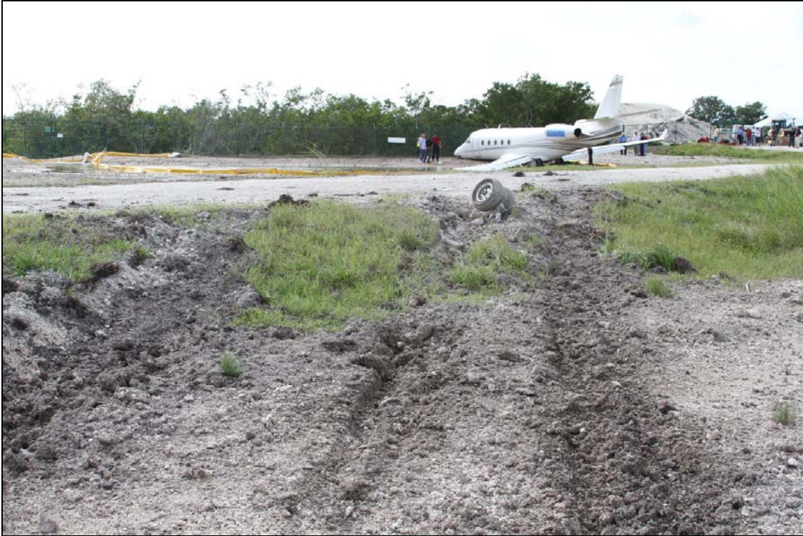
Image 2: Nose and main landing gear witness marks (ground rutting) near terrain elevation change (due to dirt road) and location of nose landing gear. NTSB photograph.
