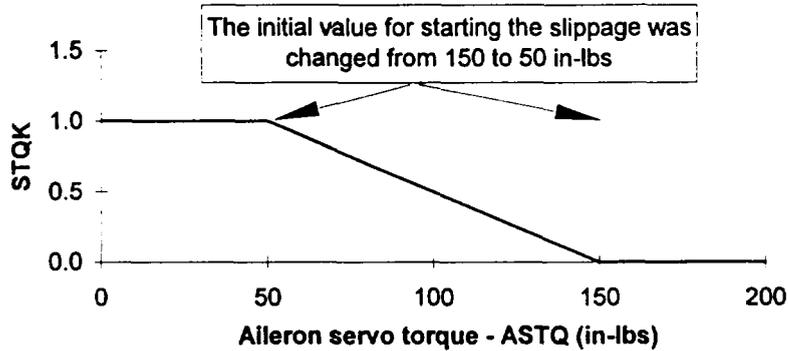
According to the above equations, the control wheel rate of deflection commanded by the autopilot is gradually reduced from its original maximum value when the servo torque reaches 50 in-lbs to zero when the demanded servo torque is above 150 in-lbs. If the initial torque for slippage is increased to from 50 to 150 in-lbs (test 1.22) the slippage occurs suddenly at 150 in-lbs.
