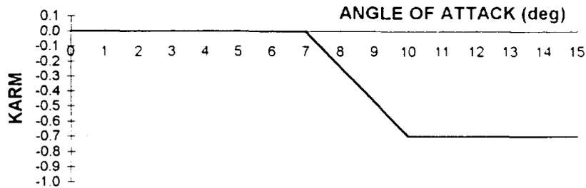
The value of 0.099 is hypothetical arm distance (in terms of wing span) from the fuselage centerline where the Delta lift and Delta drag would be acting. The Delta lift times the arm generates a rolling moment and the Delta drag times the same arm generates a yawing moment. The factor (1+KARM) takes into consideration the fact that the arm needs to be reduced when the angle of attack is increasing above 7° to reproduce the DFDR.
