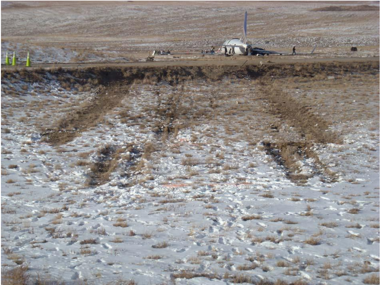
Figure 2: All Gear Tracks Reappear Beyond Taxiway Along with Engine Nacelles
