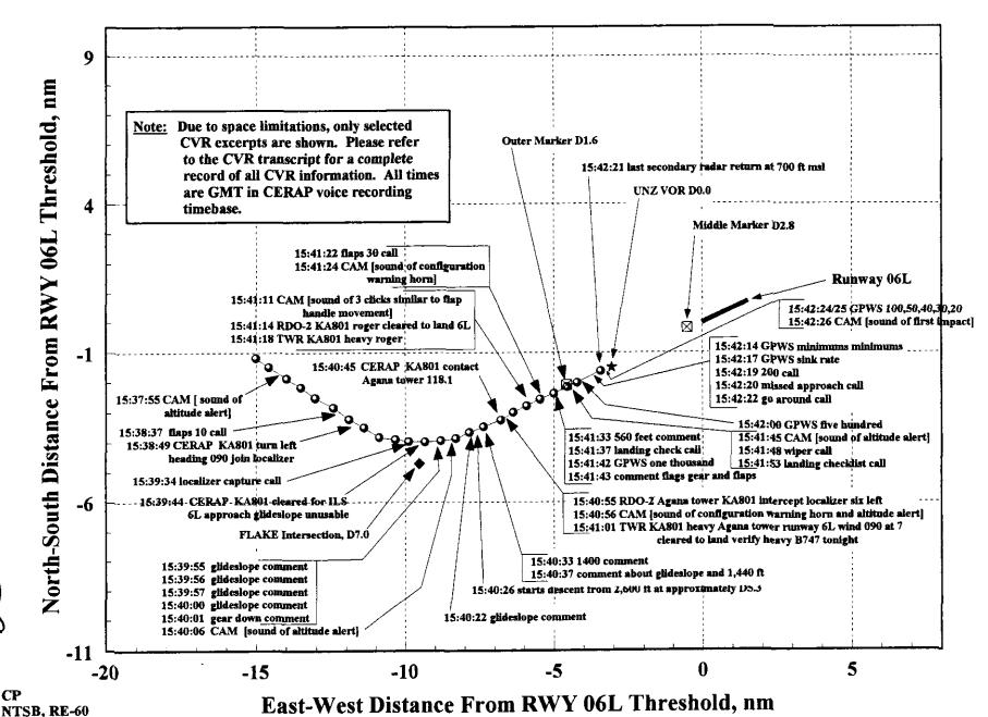
Korean Airlines B747-300 At Guam, 8/6/97 Side View Of FAA Radar Data With Selected ATC And CVR Communication Excerpts
