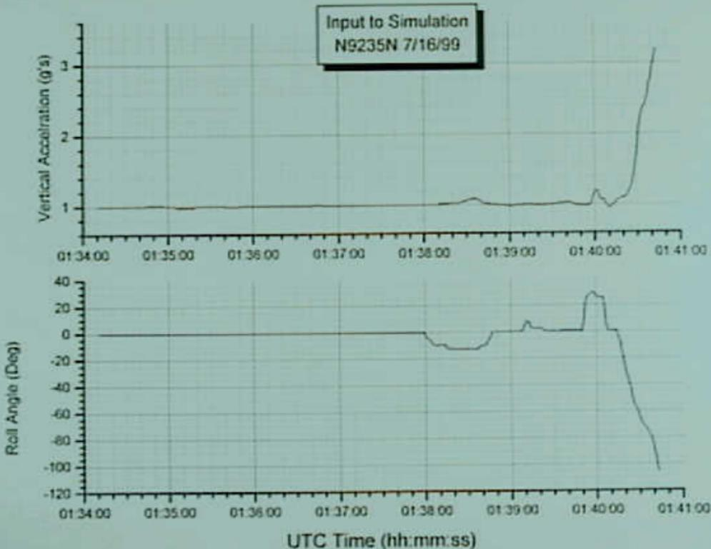
Aircraft Performance 13 - Attachment 3 - Chart 2 - Radar Data from several sources compared with Simulation Results
