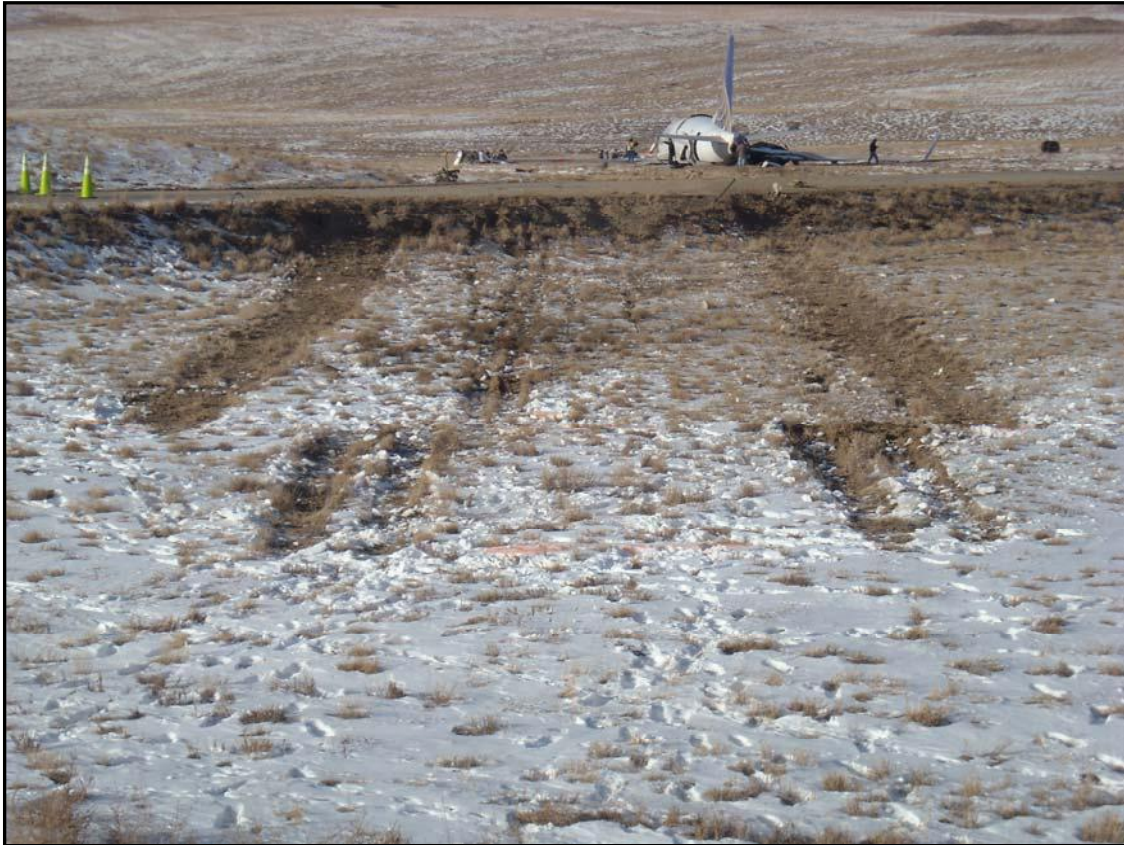
Figure 2a: Gear and Engine Nacelle Tracks Appear North of Taxiway WC
