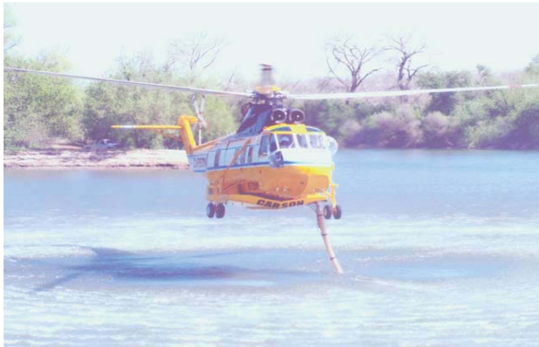
Figure 2 – Fire King Tank
