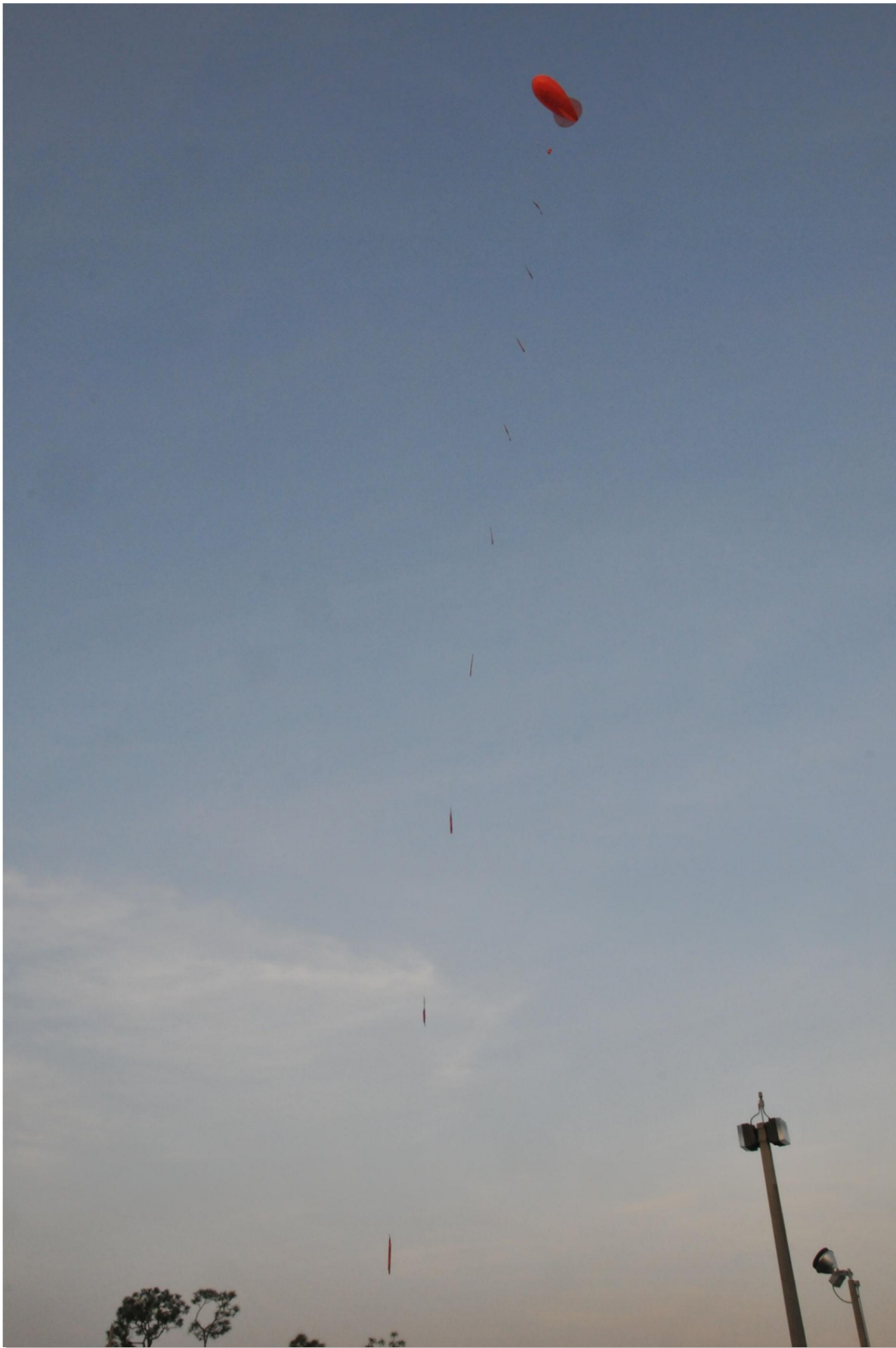
Figure 5. Image of a tethered balloon with streamers attached at various points along the tether, showing calm winds at the surface and higher winds at the balloon altitude (image provided by SAC).
