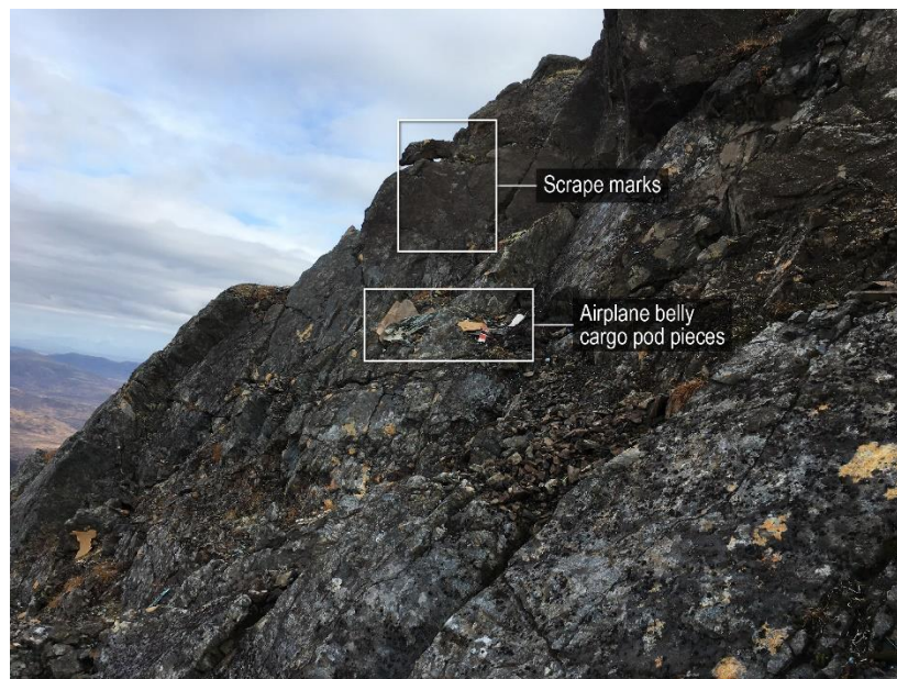
Figure 2. Photograph of the northwest (initial impact) side of the mountain ridge showing scrape marks and pieces of the airplane belly cargo pod.
