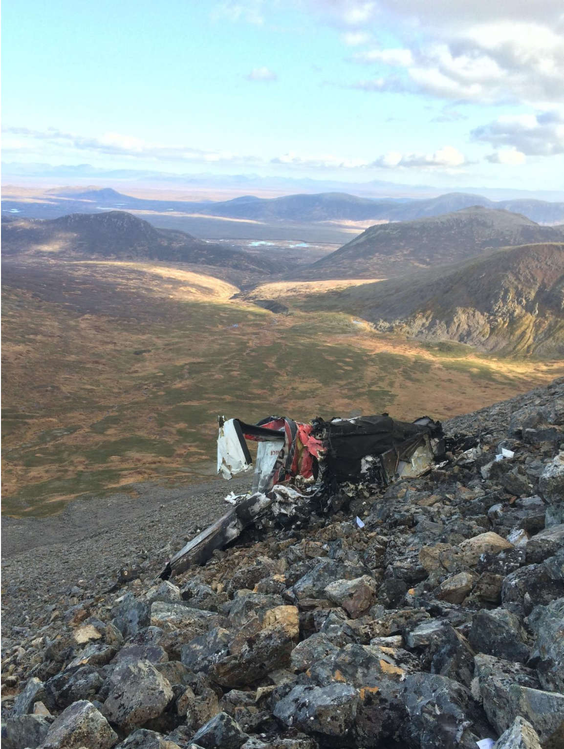
Figure 6. Separated section of empennage with vertical and horizontal stabilizers and rudder attached.
