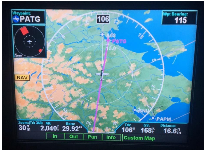
Figure 8. Photograph of the simulator’s Garmin MX 20, using the custom map function.
