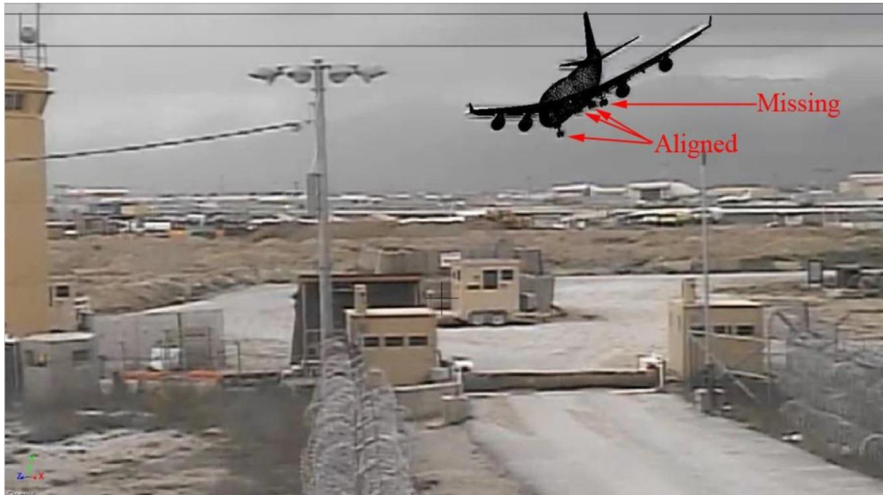
Figure 15. Still image from a security video of the accident airplane with a superimposed three-dimensional model airplane. (The model has all landing gear extended.)
