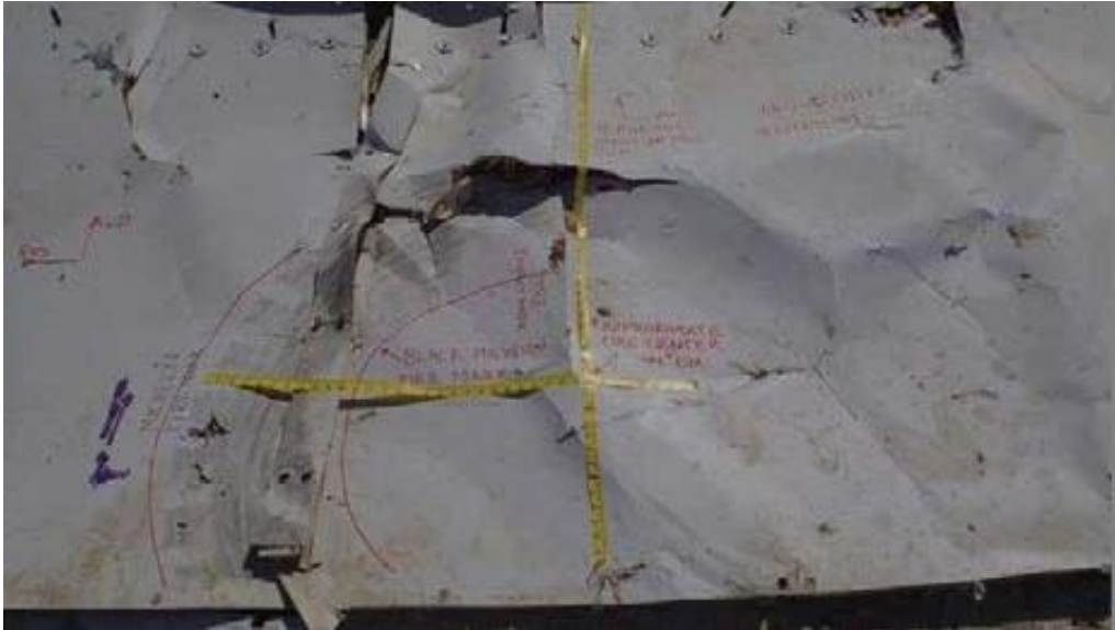
Figure 10. Photograph of M-ATV tire mark on the upper left quarter panel of the APB liner.
