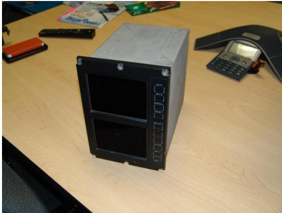
Vehicle Engine Multifunction Display (VEMD)
