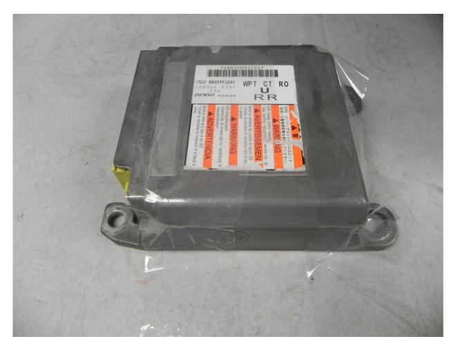
Figure 1: Denso Airbag Control Module (S/N XRR1P093725)
