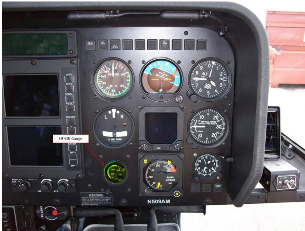
Photo4 – N509AM NF/NR gauge indicated by red arrow.
