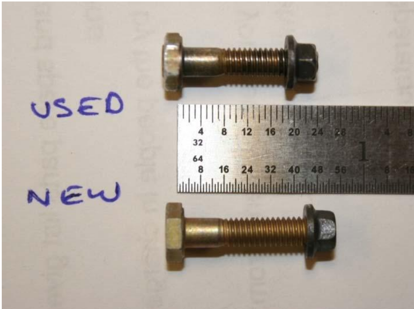
Photo 3 new and used union attachment nuts and bolts, with the nuts tightened by hand.
