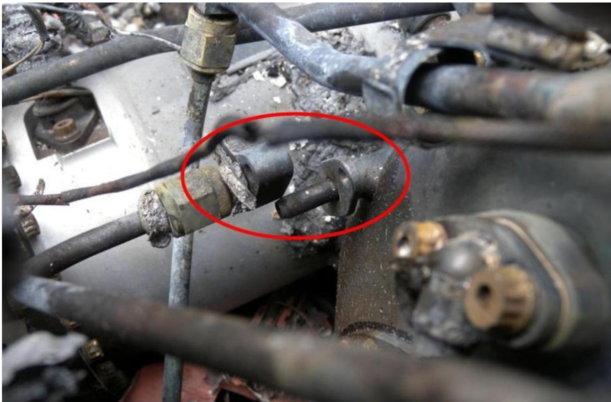
Photo 1 engine at accident site, fuel union had become detached from the flange on the compressor case
