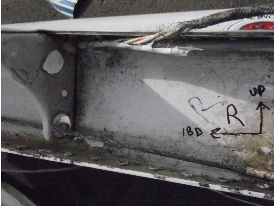
Photo 4 - Right Aileron Drive Cable at Balance Cable Pass-Through
