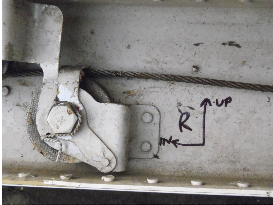
Photo 6 - Aileron Drive Cable at Outboard Balance Cable Pulley
