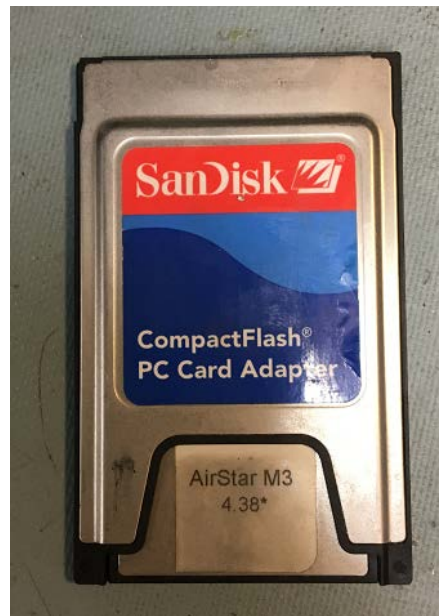
Figure 4. Compact flash card from Satloc M3 CPU.
