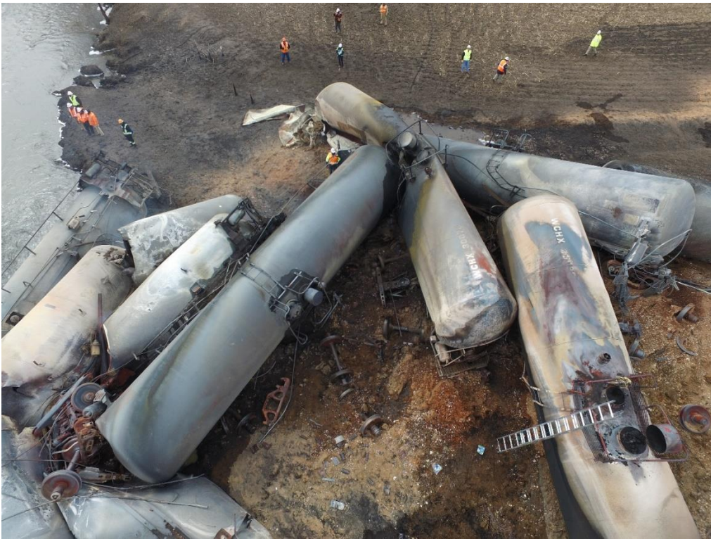
Figure 4 – Overhead of damaged cars, Jack Creek is to the left
