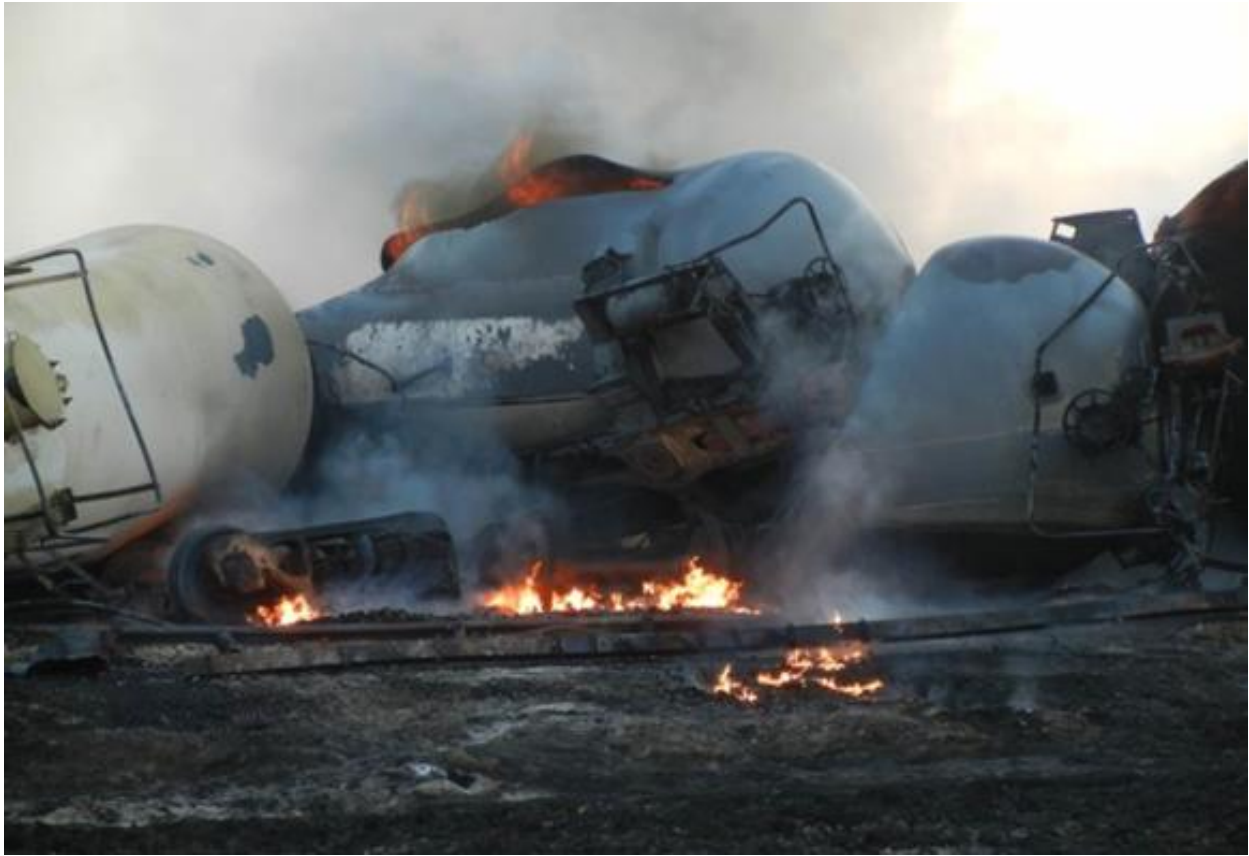
Figure 4. Derailed tank car with large thermal tear.
