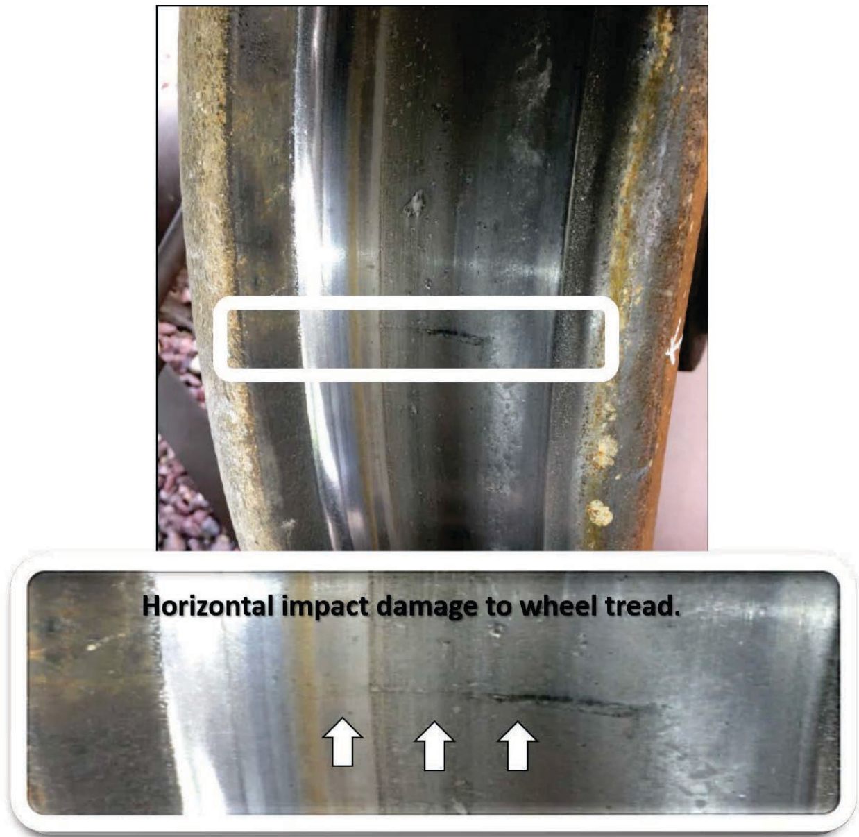
Figure 5. Wheel tread impact damage on TCBX 198115.
