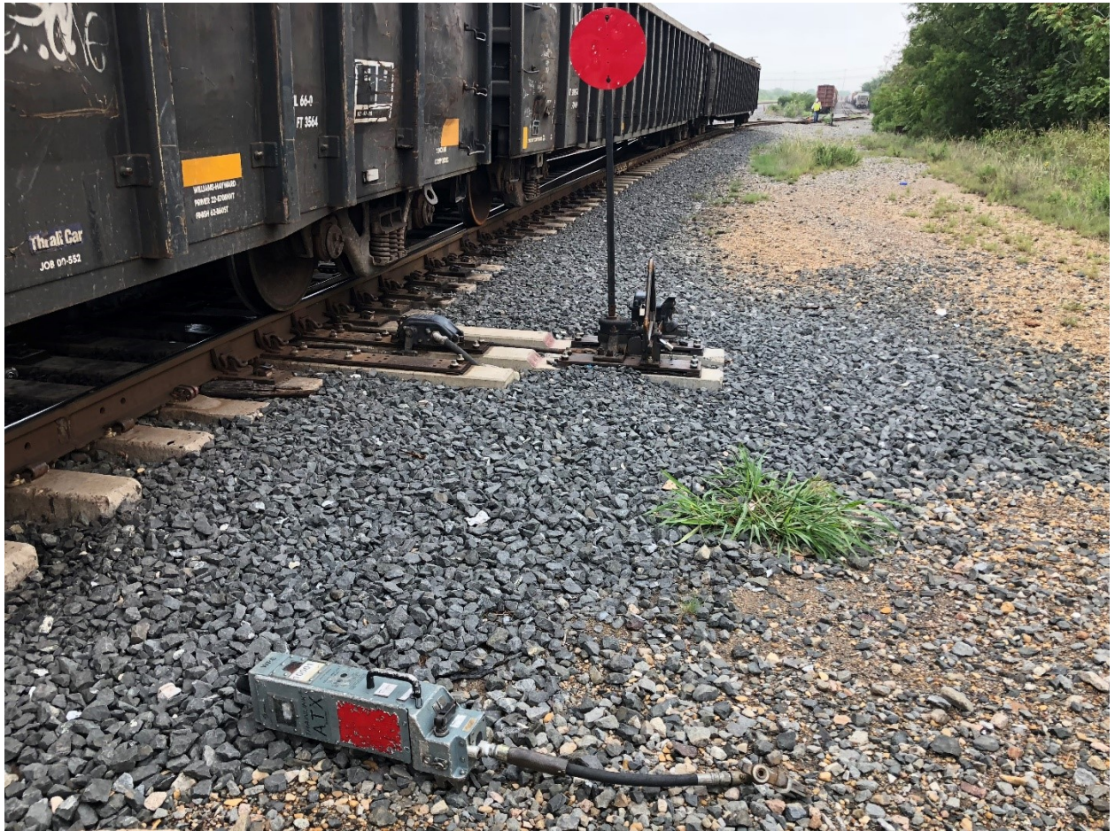
Figure 2. The accident train at the misaligned switch.
