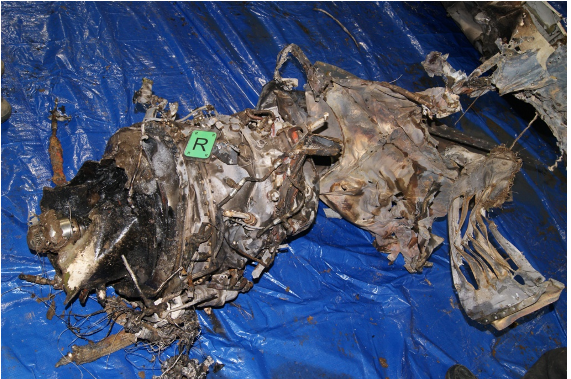
Photo 8 – View of right engine after recovery from accident site
