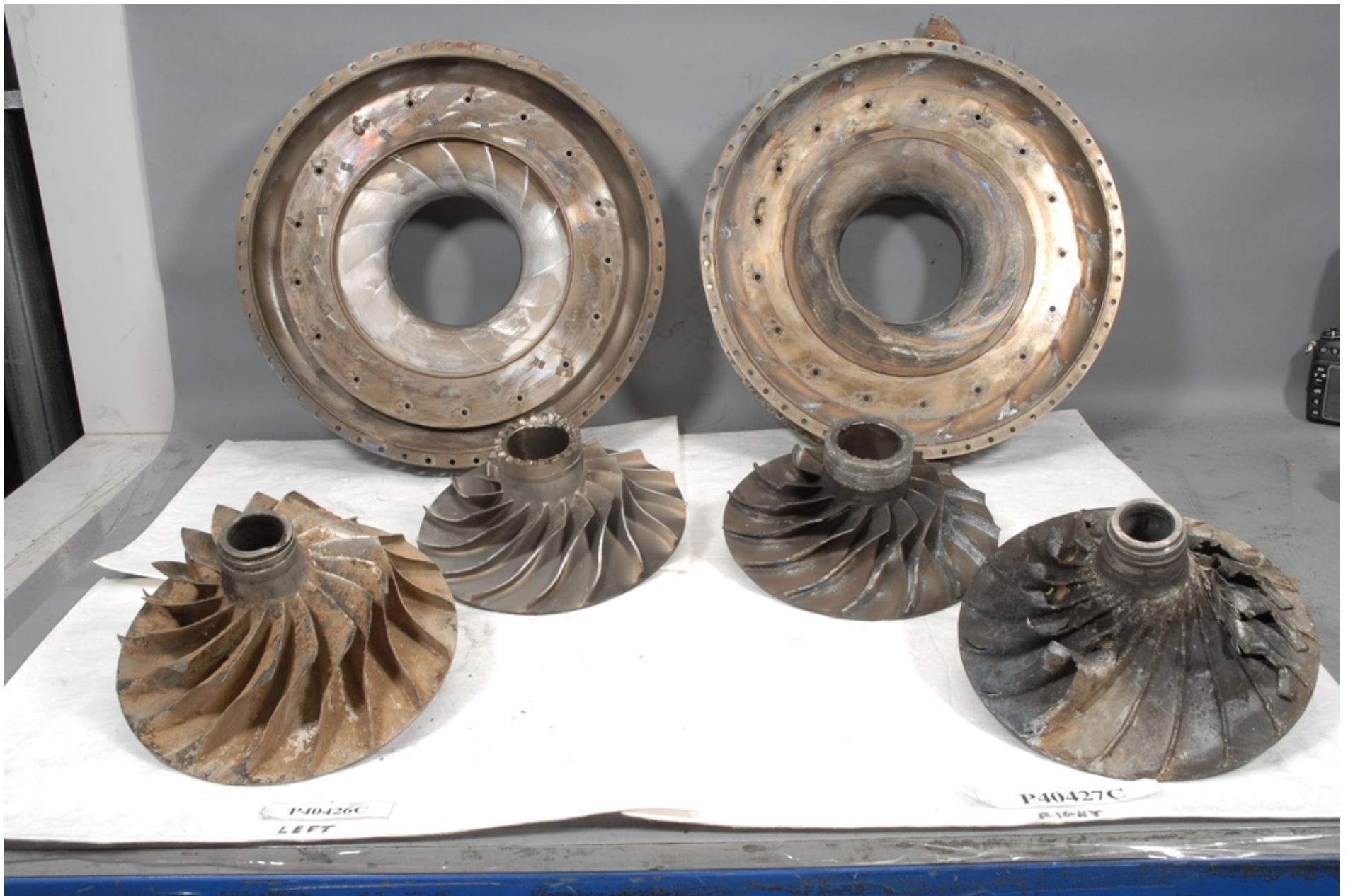
Photo 11 – Left and right engine compressor stages and compressor housings (Honeywell photograph)
