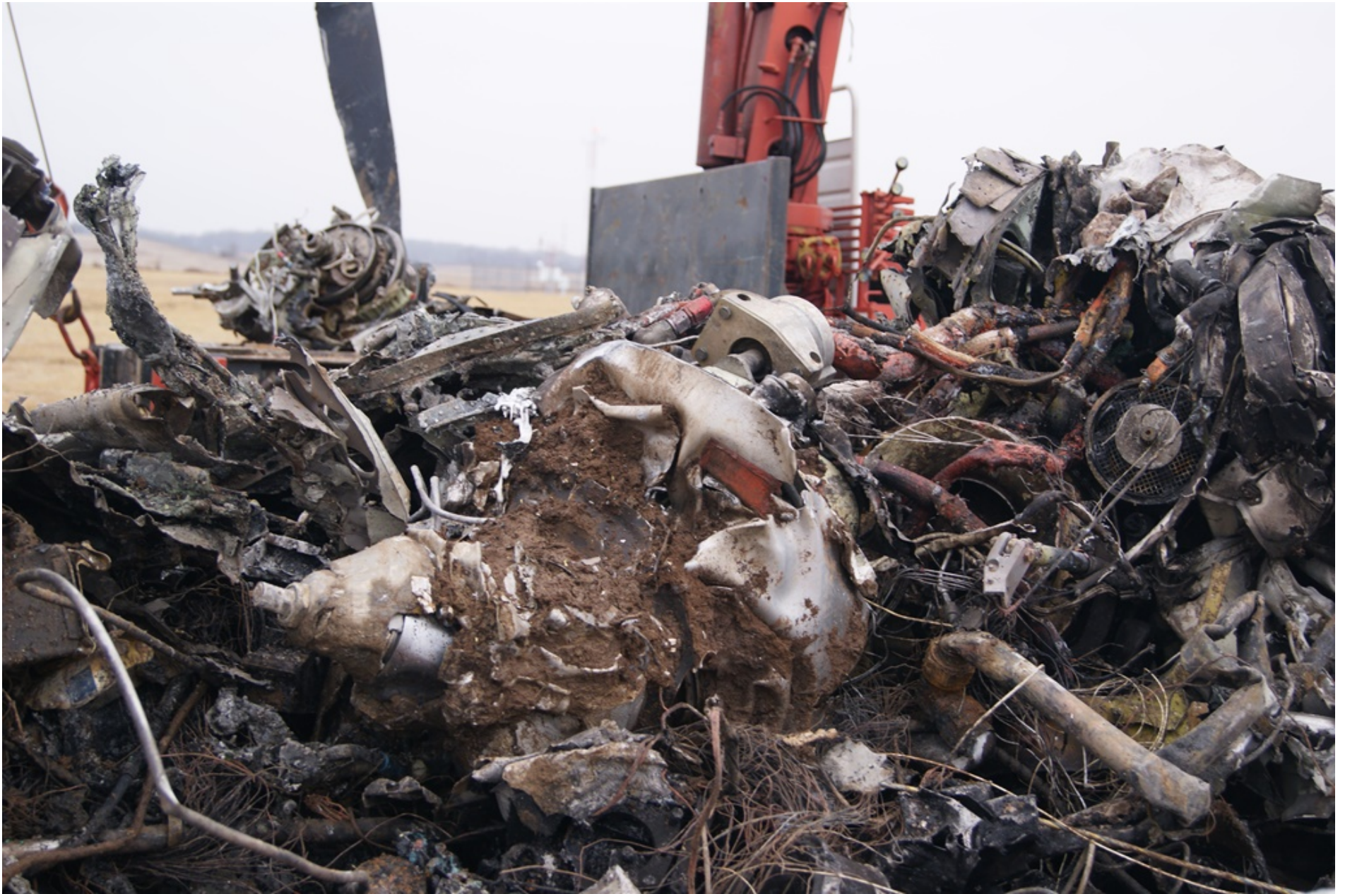
Photo 7 – View of left engine after recovery from the accident site
