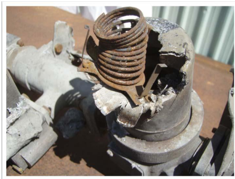
Figure 5 View of filter assembly “B” showing the fracture surface and thermal damage to the filter housing
