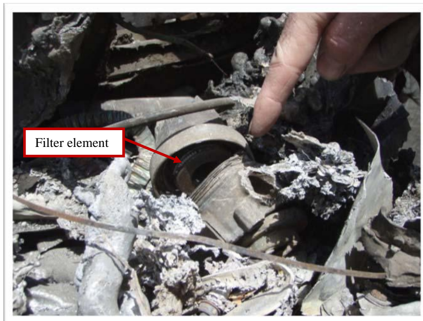
Figure 2 View of the fuel filter assembly identified as filter “A” as found within the storage bag.
