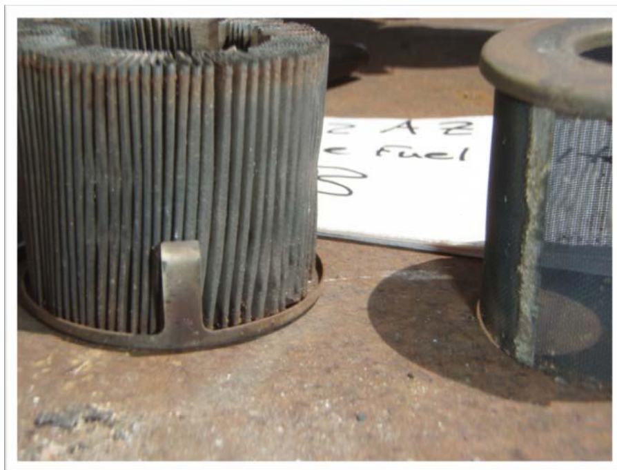
Figure 7 Close up view of the filter element “B” after being removed from the filter housing
