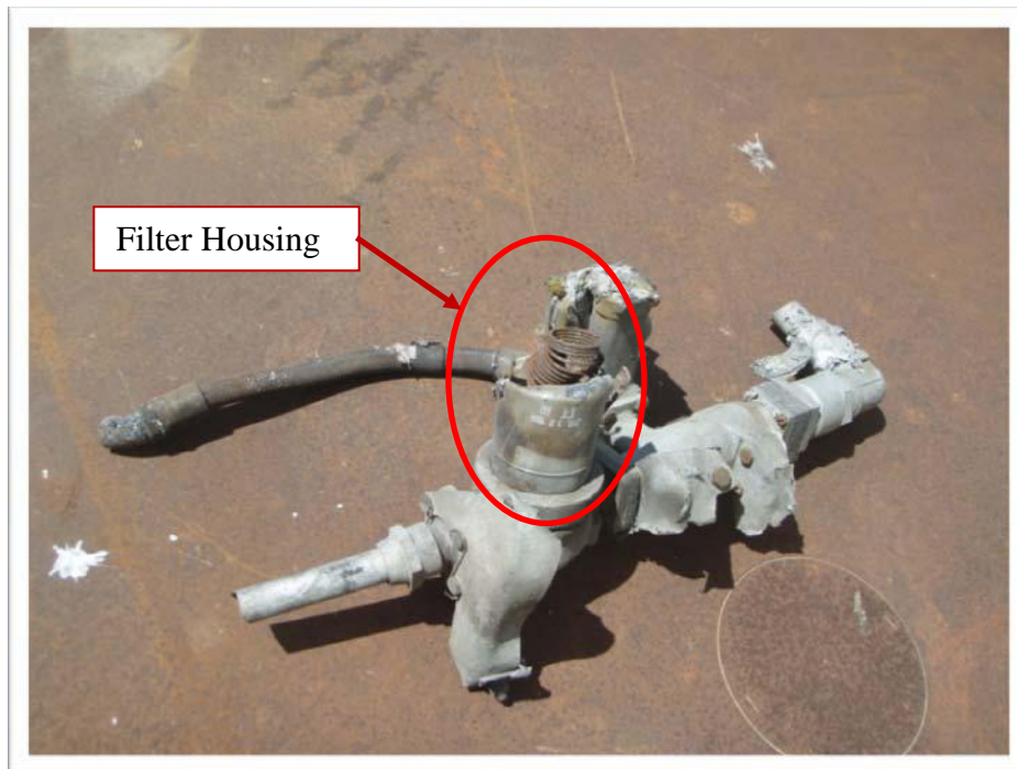
Figure 4 View of the fuel filter assembly identified as filter “B” as found within the wreckage.
