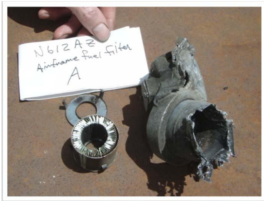
Figure 3 View of the fuel filter assembly identified as filter “A” showing the filter element removed from the filter housing
