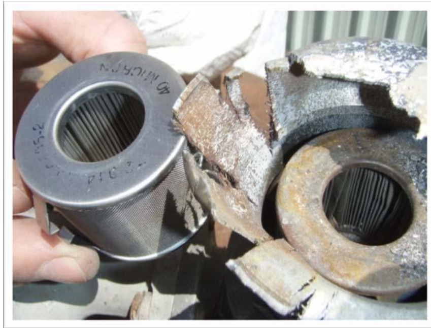
Figure 6 View of filter assembly “B” showing a comparison of the accident filter assembly to a new 40 micron filter element.
