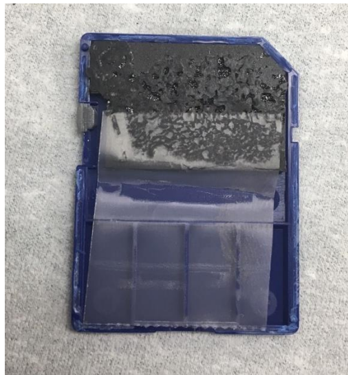
Figure 10. The silicon memory chip interfaced with a SD card package prior to a readout attempt.
