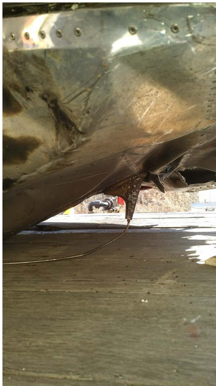
Photo 5 – Right underside of fuselage showing damaged antennae.
