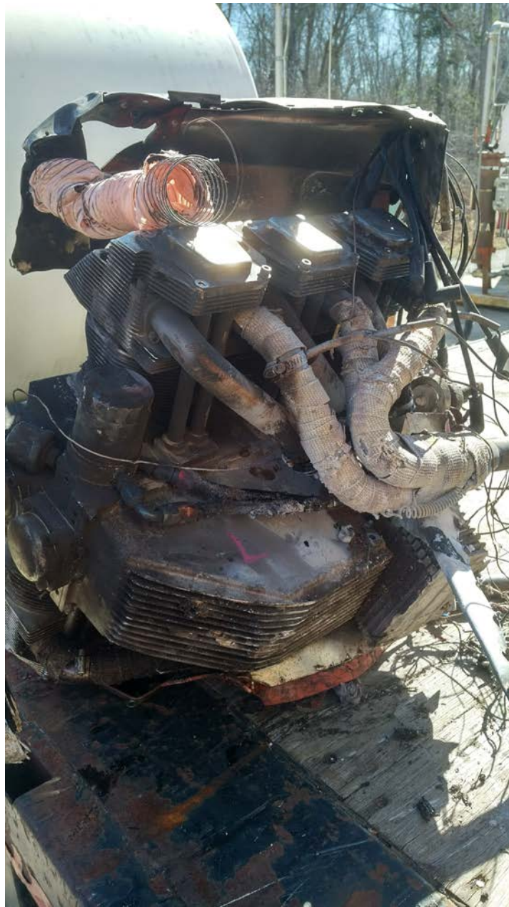
Photo 8 – Left side of engine showing damage.
