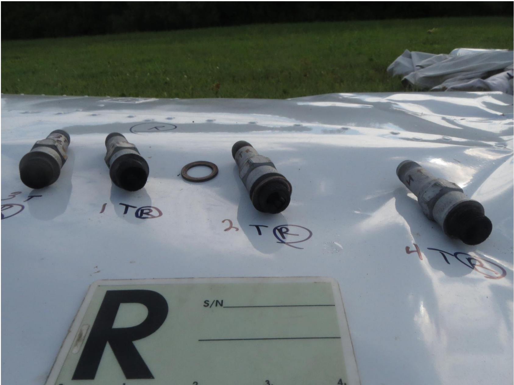
Photo 6 – Four Top Right Spark Plugs with Carbon Signatures
