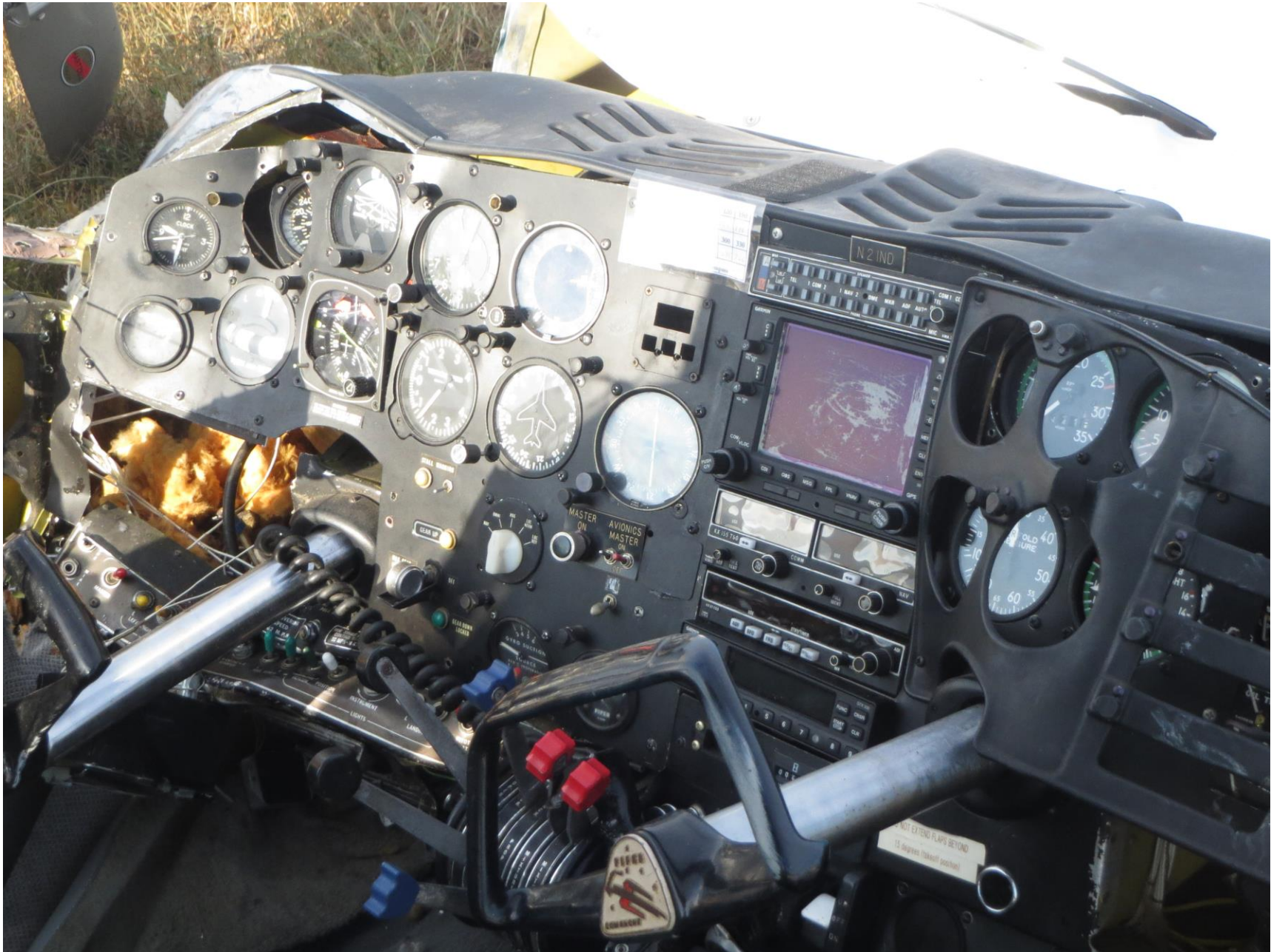
Photo 4 – Instrument Panel, Control Columns, Throttle, Propeller and Mixture Levers
